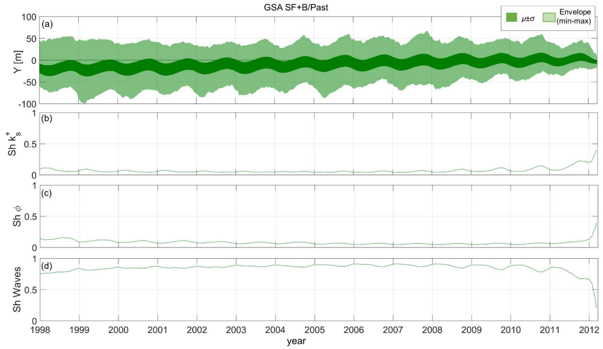
Figure 6.5. Global Sensitivity Analysis results for the ‘past scenario’, including time series of: (a) the ensemble simulated shoreline positions from 1998 to 2012; and Shapley Effects of the ShoreFor parameters (b) k_s^+ and (c) \Phi , and (d) wave chronology.
