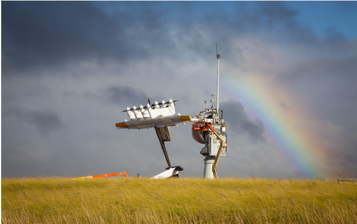
Figure 1.1 Makani's M600 AWE system. Source: Alphabet Inc [6].
