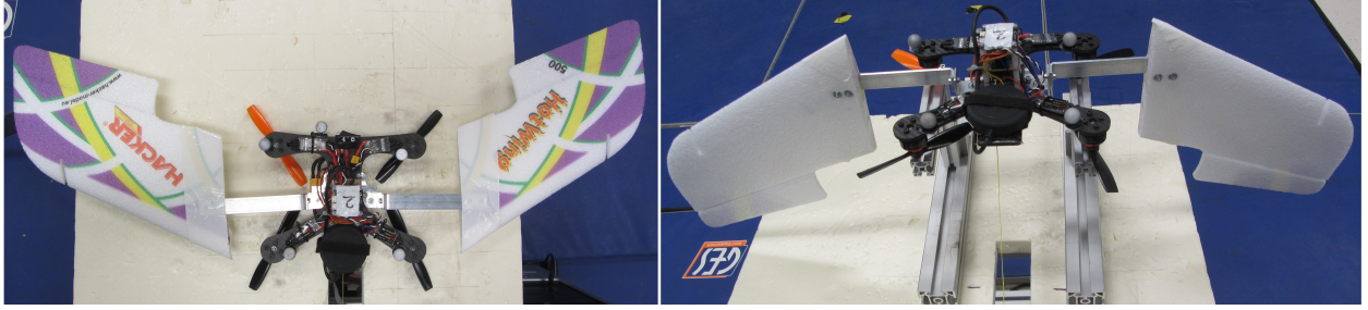
Figure 2.3 Examples of fixed configuration between the wing and the drone. Left figure corresponds to \alpha_D = 0 , and right figure corresponds to another configuration where \alpha_D = \pi/2 .
