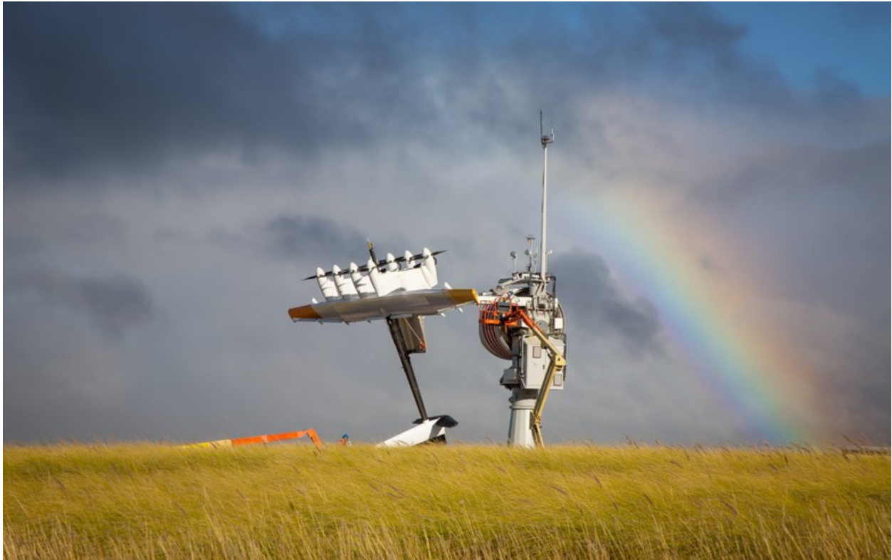
Figure 1.1 Makani's M600 AWE system. Source: Alphabet Inc [6].
