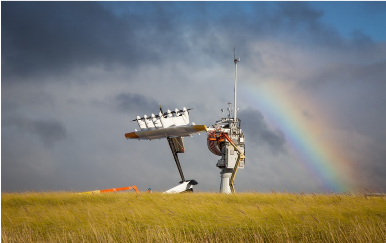
Figure 1.1 Makani's M600 AWE system. Source: Alphabet Inc [6].
