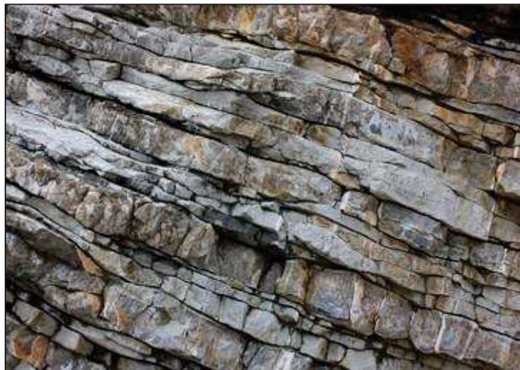
*Figure 1.21: Example of a highly fractured rock showing two fractures sets (from shutterstock.com).*
