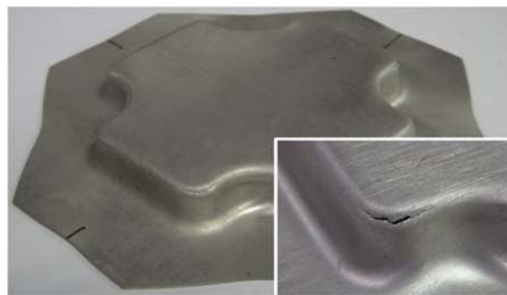
Figure 5.38: Example of fractured cross-shaped blank sheet of AZ31B [Lee15].
