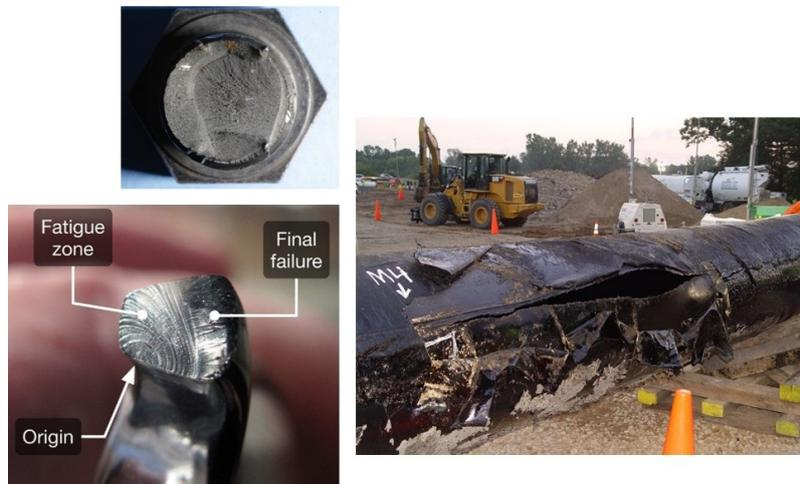
Figure 1.0.1: Examples of fatigue fracture surface and a pipeline leak. Font: NTSB 2010
