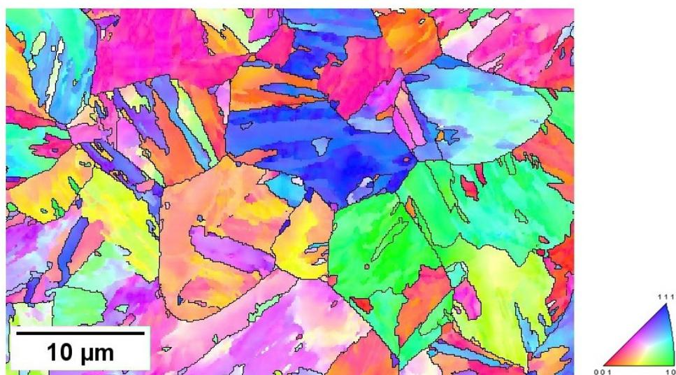
Figure 4.1.2: Inverse Pole Figure of a representative zone showing absence of any preferential texture in the WQ material
