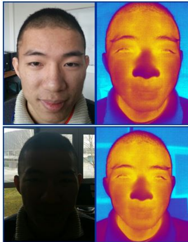
FIGURE 2.21: Thermal image is more robust against various illumination conditions than visible one
