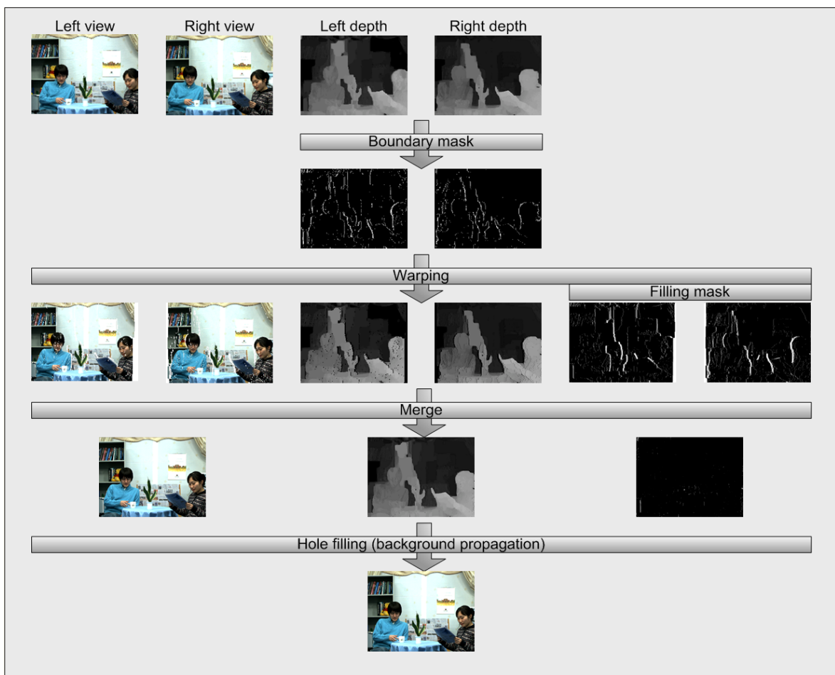
Fig. 3.2 Flow diagram for View Synthesis Reference Software (VSRS) 1D mode [9]
