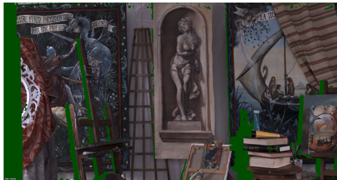
Fig. 5.6 Example of large holes (in green) in the Technicolor painter sequence with a baseline = 21cm.
