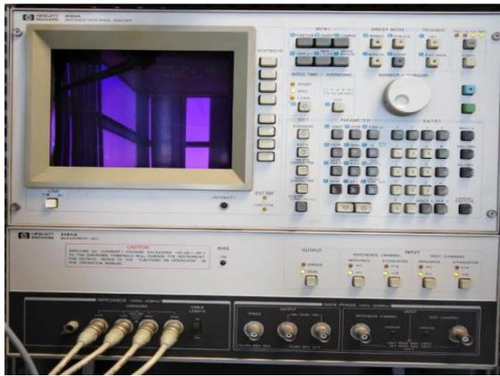
**Figure II. 9:** The Hewlett-Packard 4194A impedance meter used at the LPCA laboratory
