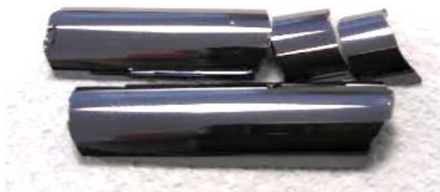
Figure I.8 Image of lead sulfide thioarsenate glasses synthesized via classical quenching method.
