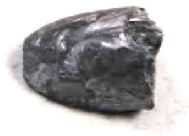
**Figure I.9** Image of the crystal dufrénoysite Pb<sub>2</sub>As<sub>2</sub>S<sub>5</sub> synthesized in LPCA laboratory.
