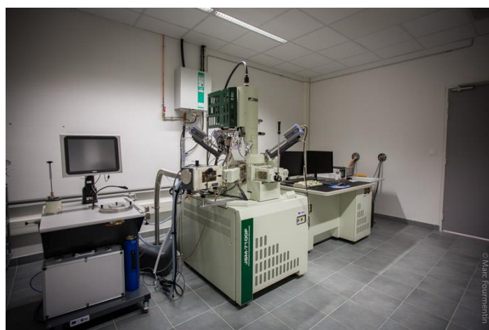
Figure I.10 The scanning electron microscopy (SEM), available at LPCA, used to examine the morphology of the synthesized samples and estimate their composition through EDX.
