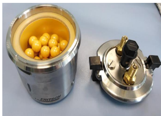
Figure I.7 Pulverisette 7 premium line used in our LPCA laboratory.
