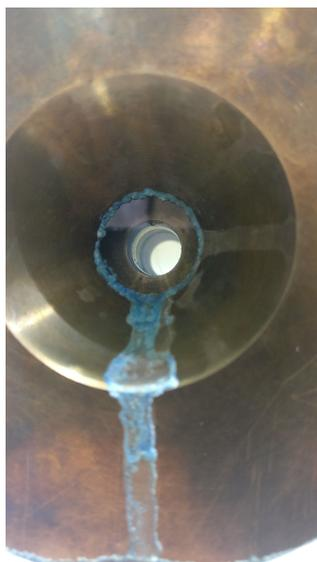
**Figure 14:** The high pressure cell used for SANS, zoomed at the saffire windows where the beam is transmitted. The picture shows the leakage of material from the windows.
