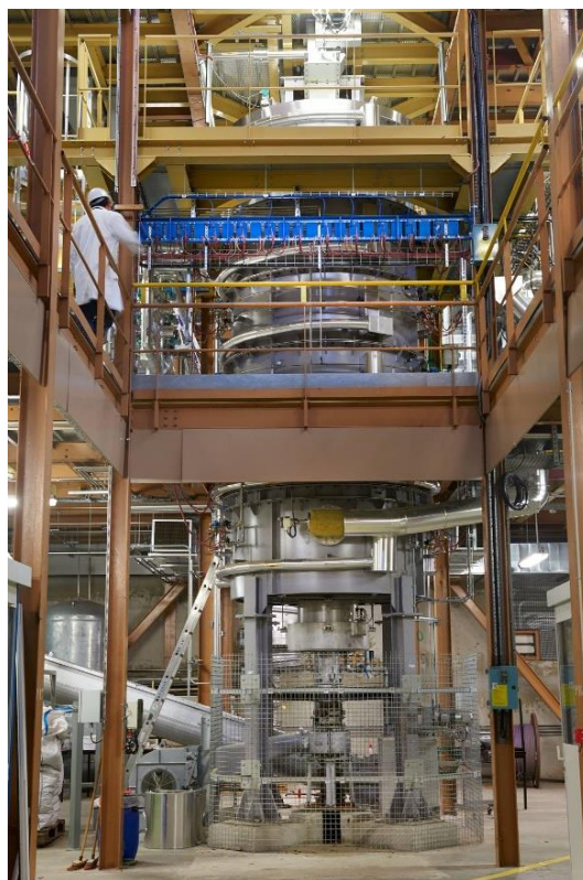
Figure 47- Photo du four de torréfaction CENTORRE (Dominique GUILLAUDIN/CEA (Malverpix No Comment Studio)).
