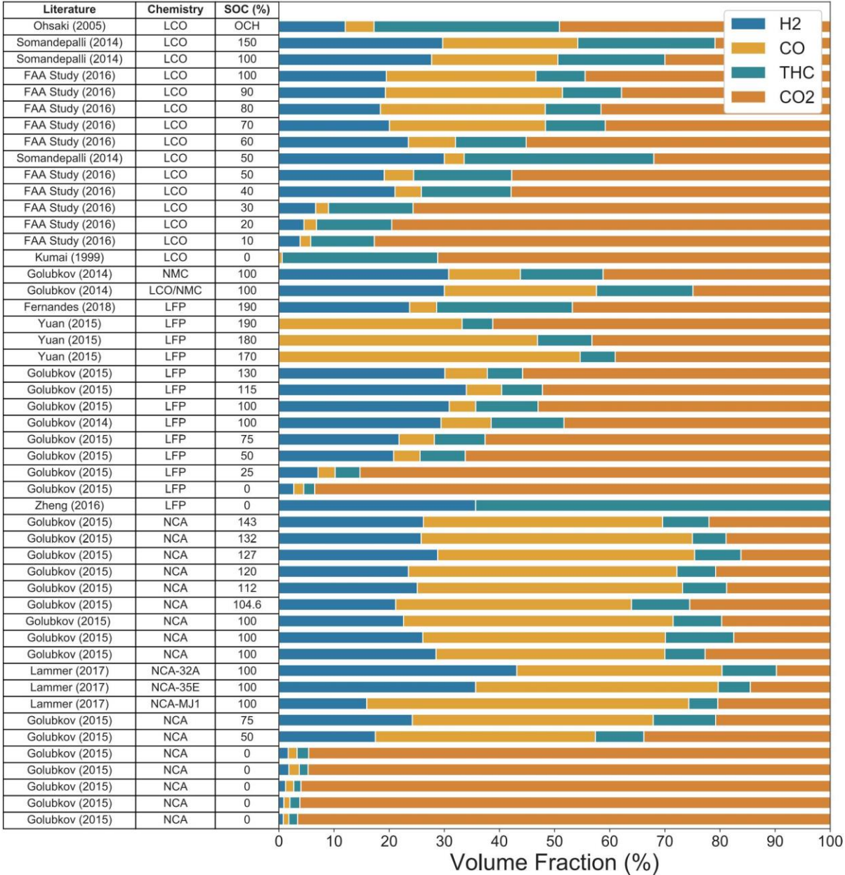
Figure 30: Battery vent gas species compositions from literature [123].
