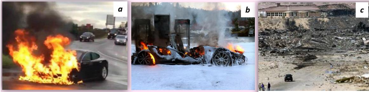
Figure 24 : a) Oct 2013 - A Tesla Model S electric car on fire after a piece of debris hit the battery pack while the car was on the highway causing cells to short circuit and go into thermal runaway; b) Jan 2016 – A Tesla Model S burns to the ground while fast-charging at the Sundebru supercharger in Gjerstad, Norway; c) Remains of the UPS Boeing 747 cargo plane that crashed in 2010 [Photo credit: EPA]
