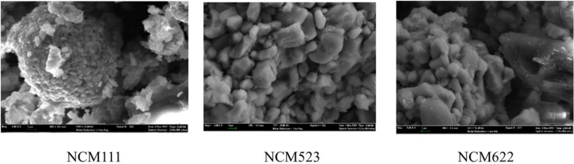
Figure 31: Vent particles (5kx) from the thermal runaway of 3 different NMCs technologies [110]
