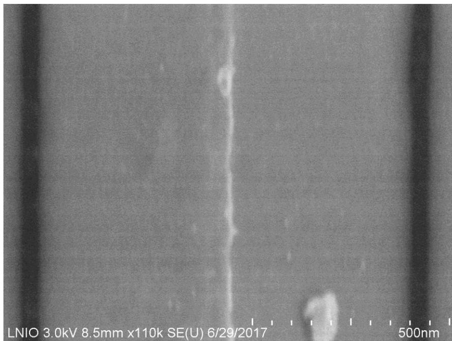
Figure 2.6. SEM images of Si surface after mask layer removing. The mask layer thickness is around 30nm, and the etching time is 1.5 hours to remove it after W-structure formation.
