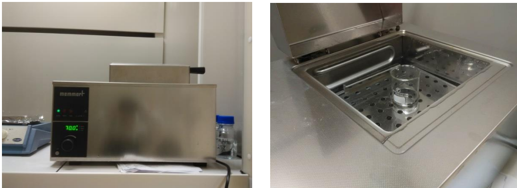
Figure 2.7. Water bath is to support a constant temperature environment.
