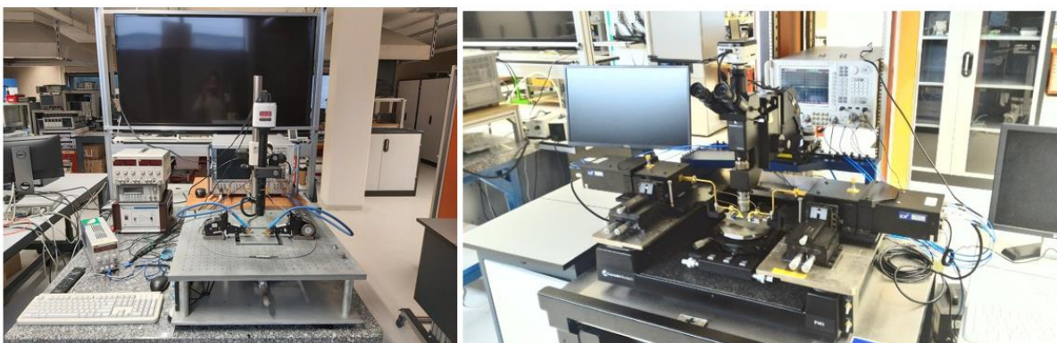
Figure 58 : Measurement Bench in XLIM, Left 10 MHz to 67 GHz, Right 75 GHz to 105 GHz
