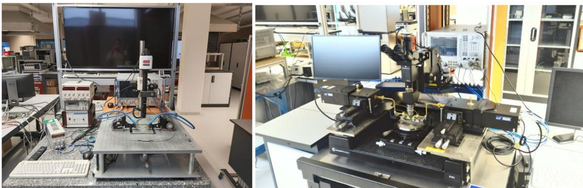
Figure 58 : Measurement Bench in XLIM, Left 10 MHz to 67 GHz, Right 75 GHz to 105 GHz
