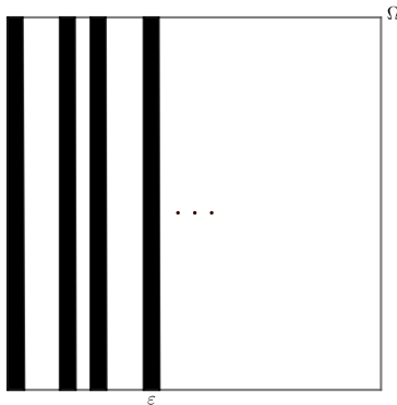
Figure 1.8: A layered material with conductivity matrix \begin{pmatrix} a_0 & 0 \\ 0 & \tilde{a}_0 \end{pmatrix} in the white region and \begin{pmatrix} a_1 & 0 \\ 0 & \tilde{a}_1 \end{pmatrix} in the black region, given conductivities a_0, a_1, \tilde{a}_0, \tilde{a}_1 > 0 .
