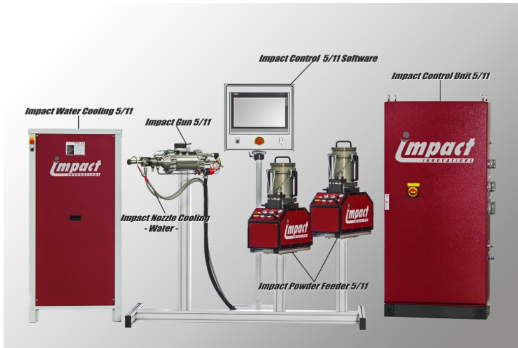
Figure 2.35 – The Impact Spray System 5/11 from Impact Innovations Company.
