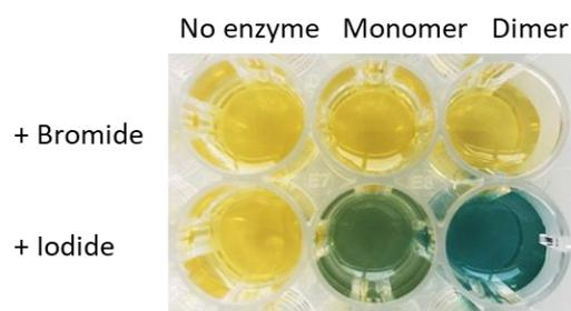
**Figure 3-6:** Thymol blue colorimetric assay of the recombinant protein Zg-VHPO3, purified as monomer and dimer batches. The assay was performed at room temperature for 1 h in clear flat-bottomed microplate wells, in presence of potassium iodide or potassium bromide. The negative control was performed without enzyme.
