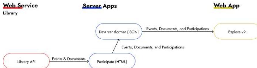
Figure 30: Back-end architecture of the second version of Explore.
