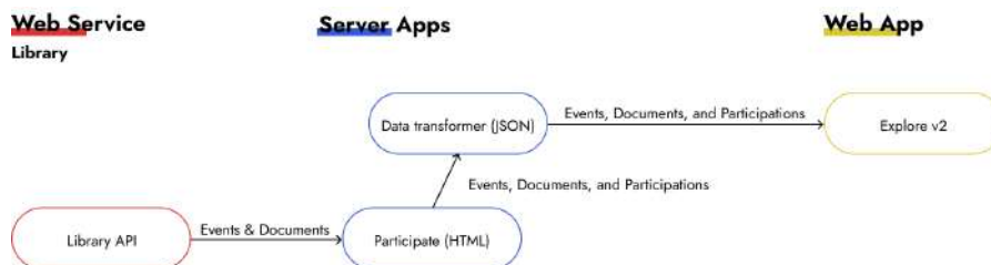
Figure 30: Back-end architecture of the second version of Explore.
