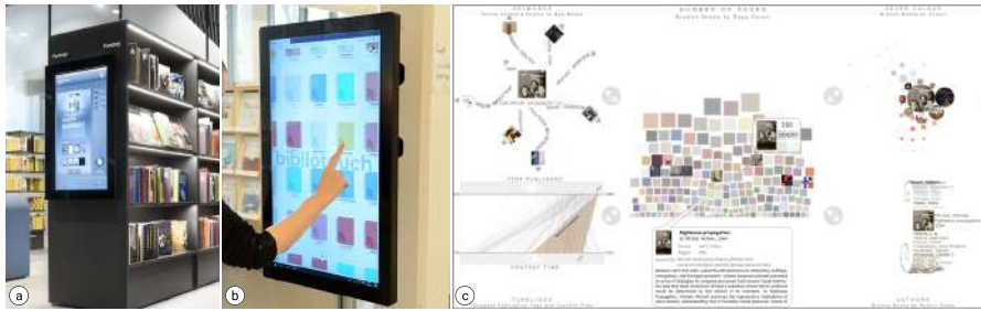
Figure 3: (a) A display embedded on a shelf at Dokk1 (b) Bibliotouch, a collection exploration tool, and (c) Bohemian Bookshelf, a serendipity exploration device
