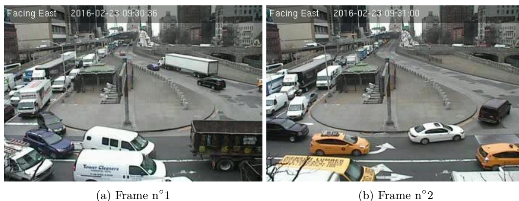
Figure 4.4 – Two consecutive frames on the WebCamT dataset. Comparing the timestamps on top of the frames, we can see that they are 24 seconds apart. Therefore, the frame rate is too low to produce any usable video.
