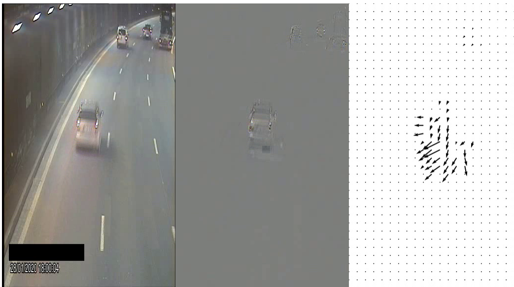
Figure 4.1 – Visualization of a frame of a video stream alongside its compressed representation. From left to right are the original RGB frame, the residual image and the Motion Vector (MV) representation. We see that only the moving vehicles generate data to be compressed. Note that motion vectors point in the opposite direction of the vehicles flow as they refer to previous frames.
