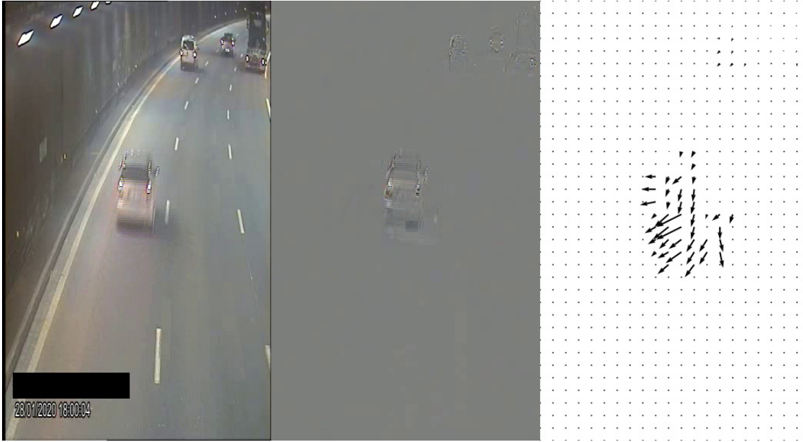
Figure 1.11 – Visualization of the original frame of a video stream alongside its compressed representation. From left to right are the original RGB frame, the residual image and the MV representation. We can see that only the vehicles generate data to be compressed as they are the only moving objects on screen. Motion vectors point in the opposite direction of the vehicles flow as they refer to previous frames.
