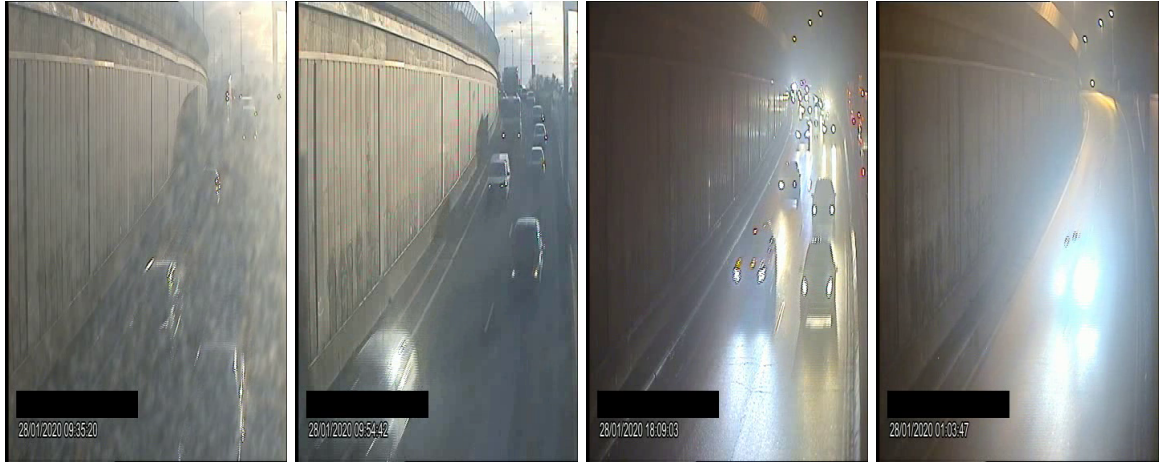
(a) Reflects due to the sun position and dirtying of the lens. (b) Typical day configuration. (c) Typical night configuration. (d) Intense illumination probably due to the car having headlights full on.
