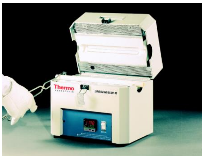
Figure 34: Image of the tubular CVD used in this work
