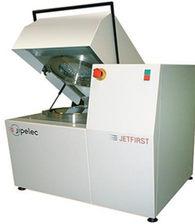
Figure 13: View of the CVD used for the growth of graphene
