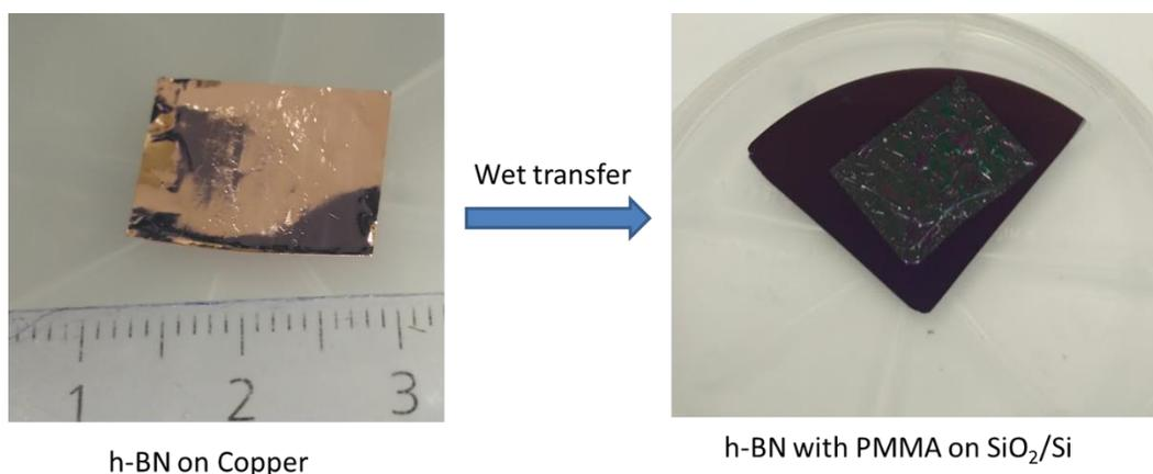
Figure 44: Image of h-BN before and after transfer
