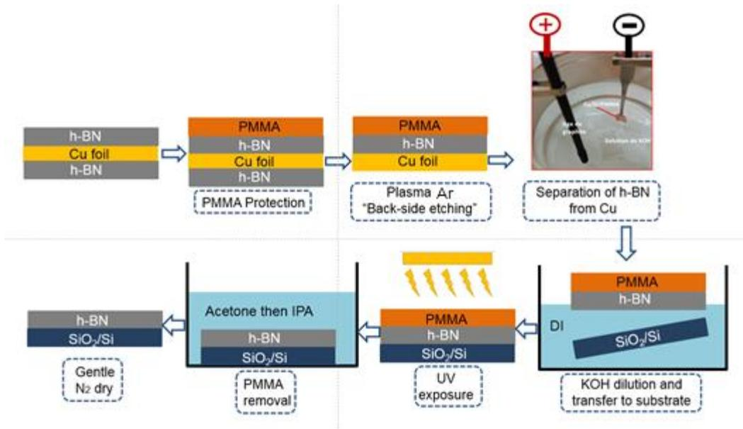
Figure 45: Schematic of the bubbling transfer process
