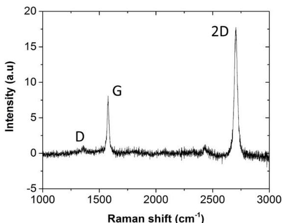
*Figure 18: Raman spectra of graphene on copper foil*
