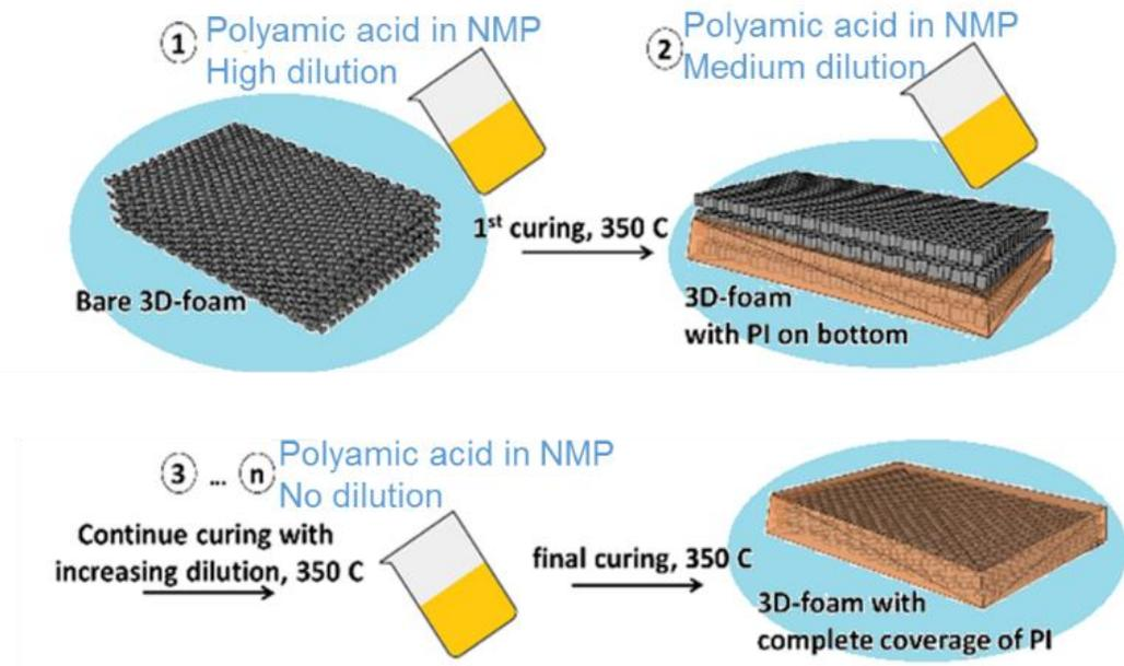
Figure 56: Schematic of the second generation film process
