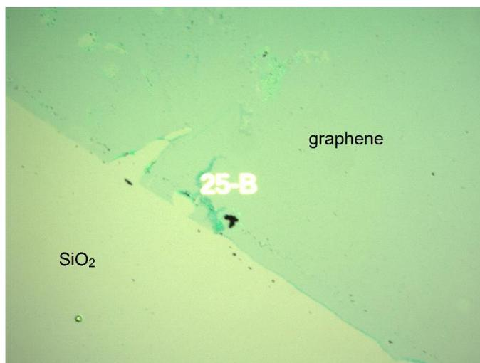
*Figure 9: Example of optical image of graphene on SiO<sub>2</sub>*
