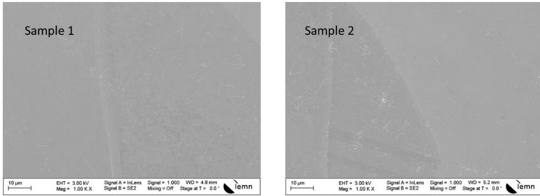
Figure 39: SEM images of h-BN on copper
