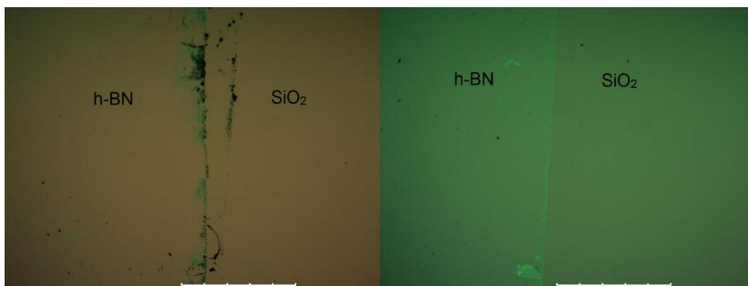
Figure 47: Optical images of h-BN (sample 1 and sample 2) transferred on SiO<sub>2</sub>
