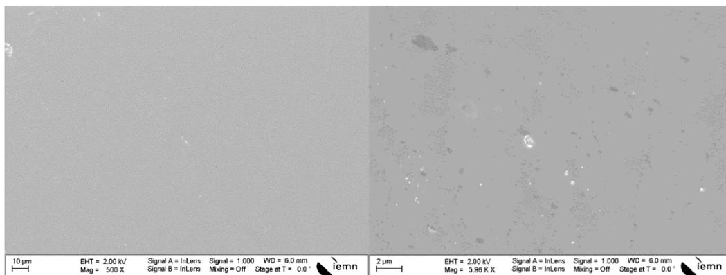
*Figure 16: SEM images of graphene on copper foil*
