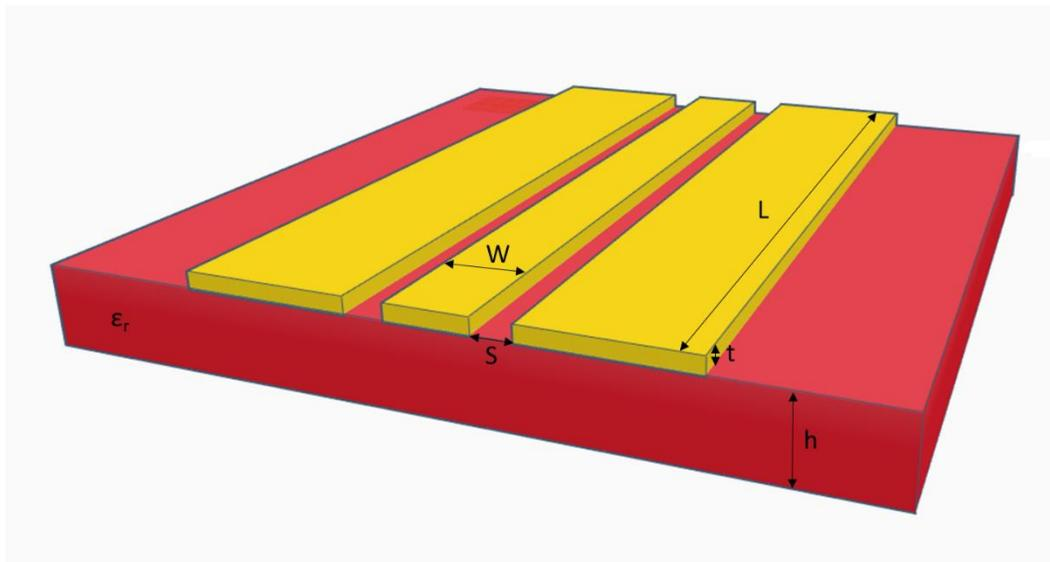
Figure 73: Schematic of a CPW transmission line
