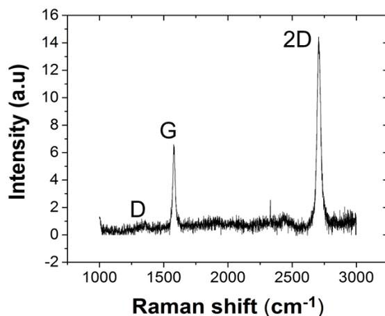
Figure 27: Raman spectra of single crystal graphene
