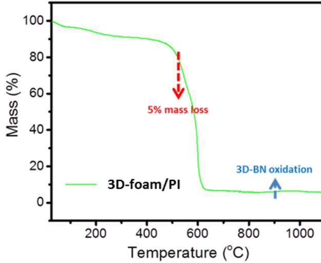
Figure 64: TGA thermal stability of 3D-BN/PI
