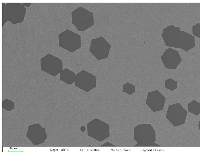
Figure 24: SEM image of single crystals graphene
