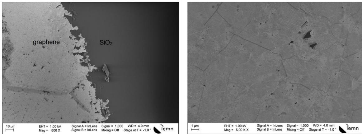
Figure 22: SEM images of graphene transferred on  $\text{SiO}_2$
