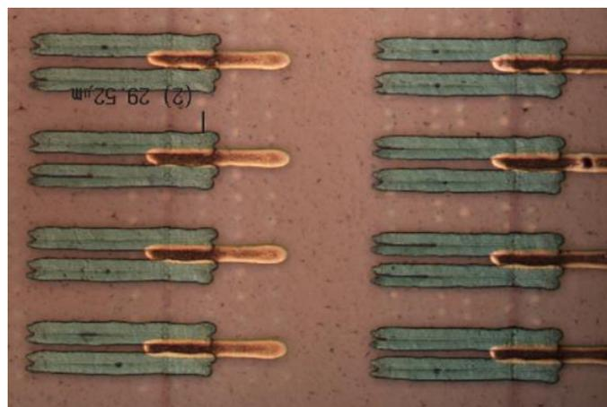
Figure 76: Optical image of the printed transistors
