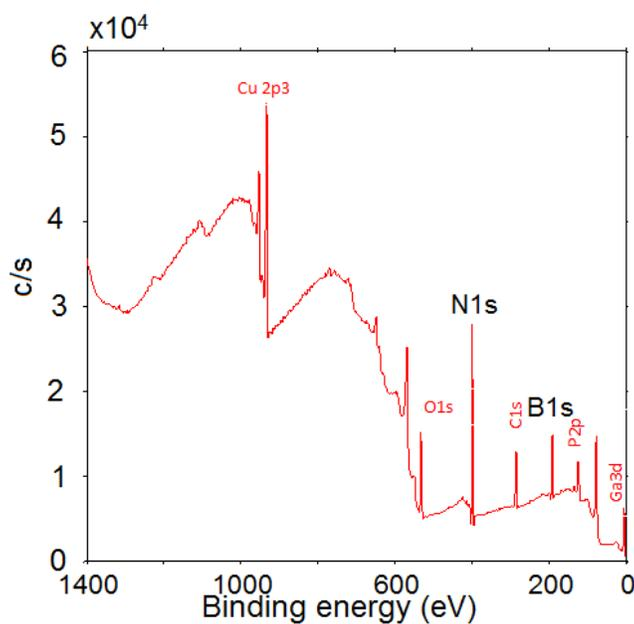
Figure 42: XPS spectra of h-BN on copper
