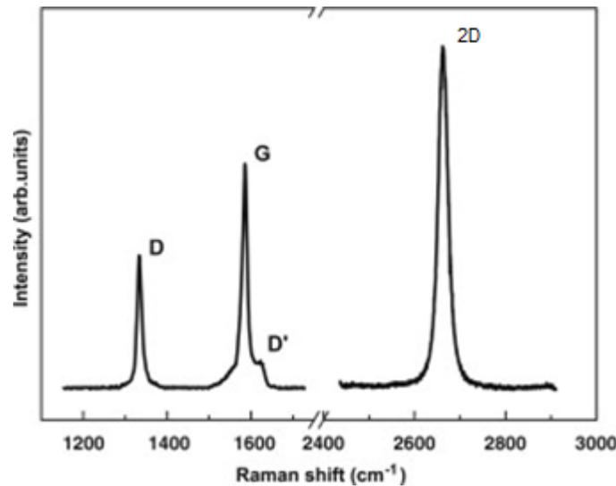
Figure 11: Example of Raman spectra of graphene[34]
