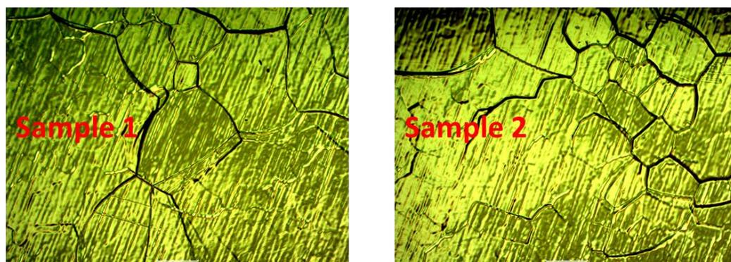
*Figure 38: Optical images of h-BN on copper*
