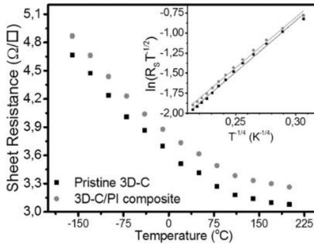
Figure 63: Sheet resistance of bare 3D-C and 3D-C/PI at a temperature range of  $-160$  to  $200$  °C (inset: fit of VRH model, that is  $\ln(R_s T^{-1/2})$  versus  $T^{-1/4}$  for both materials)
