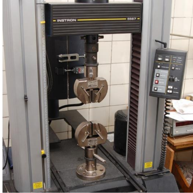
Figure 61: Set up of the stretching test using INSTRON 5567
