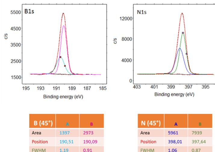
Figure 43: Peak parameters from the XPS signal
