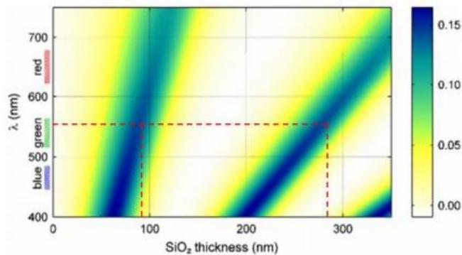
Figure 8: *Optical contrast of graphene as a function of the wavelength and the SiO<sub>2</sub> thickness*[29]
