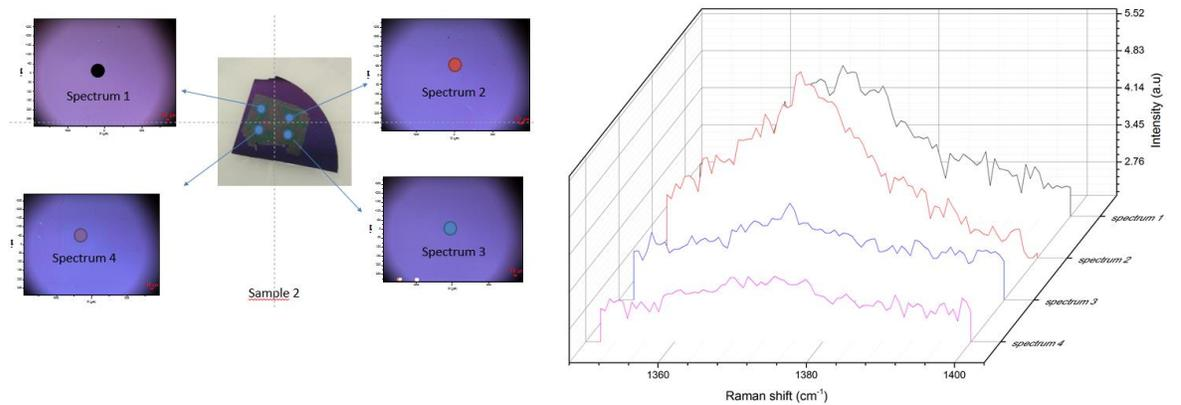
Figure 50: Raman spectrum of sample 2
