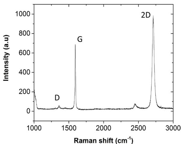
*Figure 23: Raman spectra of the 3DC foam*
