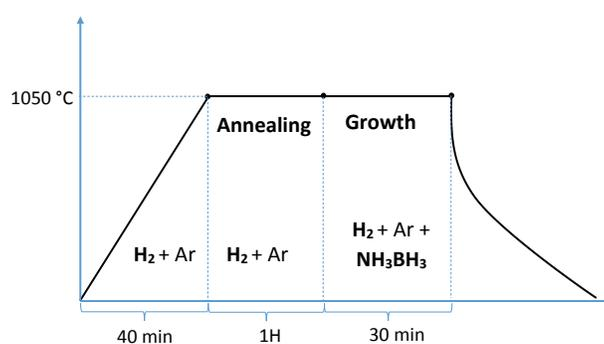
Figure 35: Schematic of the growth process of h-BN
