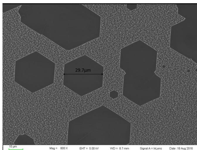
Figure 26: SEM image of single crystal graphene
