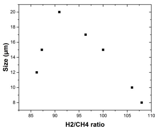
Figure 25: Average size of the grains as a function of the H<sub>2</sub>/CH<sub>4</sub> ratio
