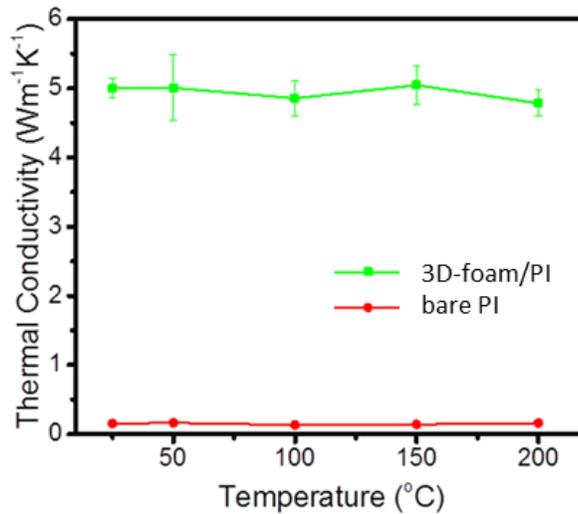
Figure 65: Laser Flash thermal conductivity result of 3D-foam/PI
