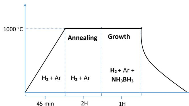
Figure 51: Schematic of the 3DBN growth process
