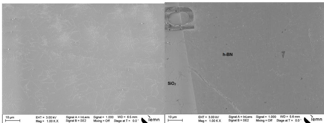
Figure 48: SEM images of h-BN (sample 1 and sample 2) on SiO<sub>2</sub>
