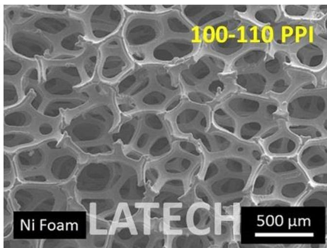
Figure 28: SEM image of the Ni foam[50]
