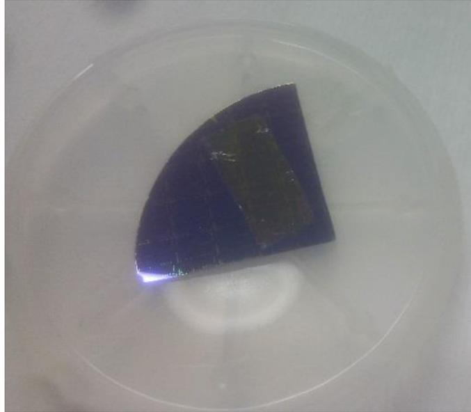
*Figure 20: Optical image of graphene with PMMA transferred on SiO<sub>2</sub>/Si*
