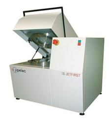
Figure 13: View of the CVD used for the growth of graphene
