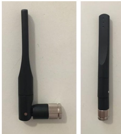
Figure II. 7: Antenne monopôle de type PSKN3-24/55 RS.
