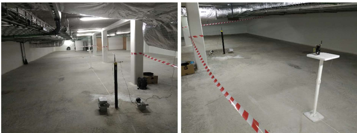
Figure V.64: Photographs of an experimentation in indoors (subbasement of the laboratory) of an integrated sensing node of the same generation than SN4, wirelessly powered by a communicating node.
