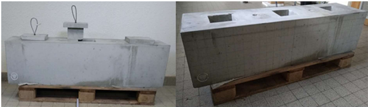
Figure III.2: Photographs of the reinforced concrete beam used to perform experiments for the McBIM research project.
