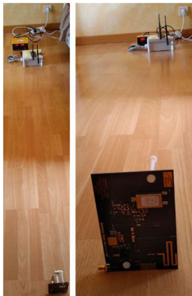
Figure V.63: Photographs of an experimentation in indoors (room) of an integrated sensing node of the same generation than SN4, wirelessly powered by a communicating node.
