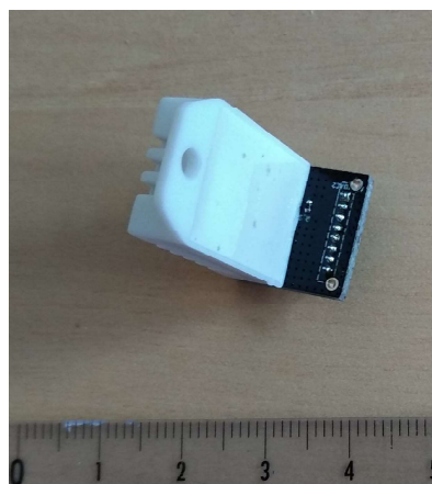
Figure V.7: Photograph of the designed and implemented daughter board interfacing the Adafruit DHT22 temperature and relative humidity sensor.
