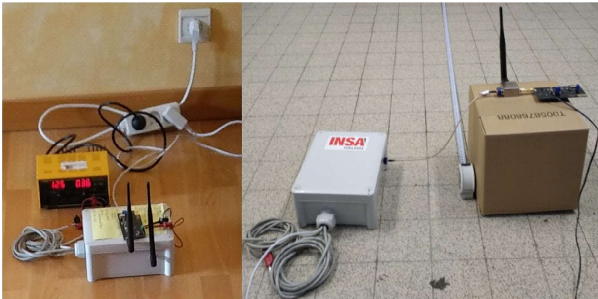
Figure IV.8: Photographs of a communicating node in various configuration: using two independent subsystems located at the same place; and using a radiofrequency circulator and a unique antenna.
