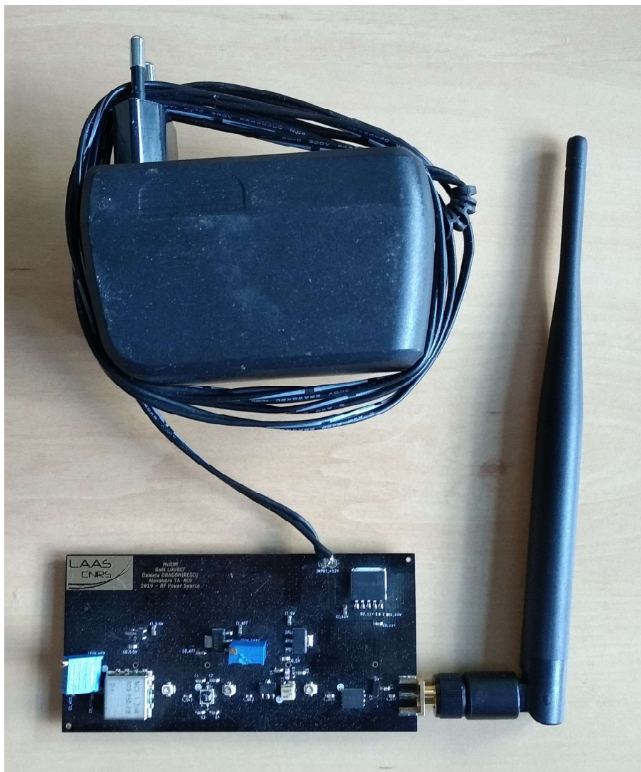
Figure IV.3: Photograph of the designed and implemented +33 dBm continuous wave radiative electromagnetic power source in the 868 MHz industrial, scientific and medical (ISM) frequency band.
