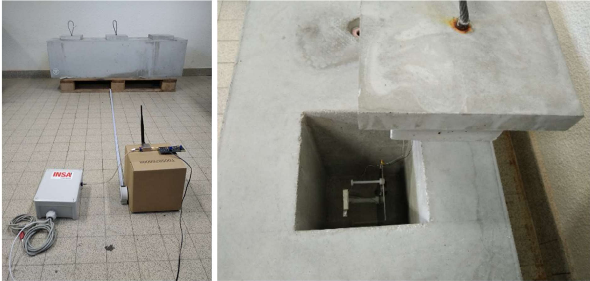
Figure V.65: Photographs of an experimentation of three integrated sensing nodes of the same generation than SN4 embedded into the reinforced concrete beam, wirelessly powered by a communicating node.
