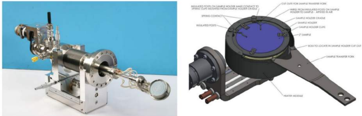
Figure 2.5: picture of multi-axis manipulator arm including the heating module (left). Schematic representation of the sample holder and transfer arm.
