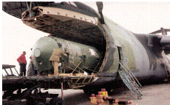
Figure 1.8 Thermionic reactor of TOPAZ II at Kirtland Air Force Base
