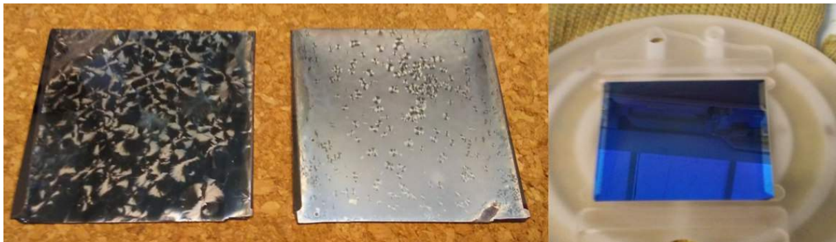
Figure 2.30: Left, sample of \text{Cs}_2\text{CO}_3 with a layer of \text{Al}_2\text{O}_3 (b) middle, sample of \text{Cs}_2\text{CO}_3 without protection (c) right, same sample just out of ALD vacuum chamber
