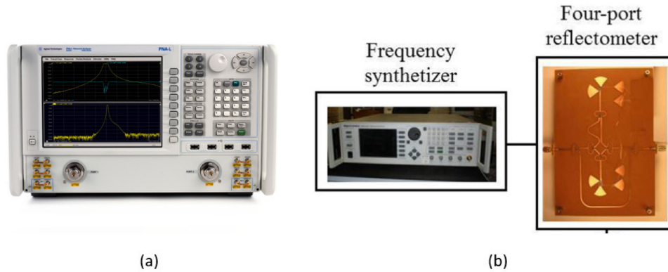
Figure I-6: Schematic of a signal generation/acquisition system: (a) VNA (b) a combination of a frequency synthesizer and multi-port based reflectometer [HAD 11].
