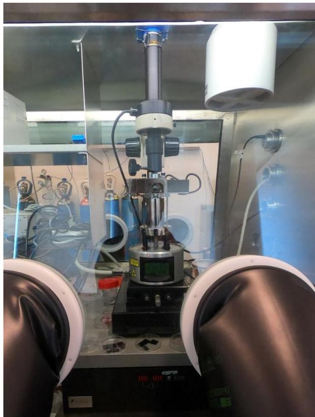
**Figure 2.9.** *Bruker Multimode AFM inside a N<sub>2</sub>-filled glovebox.*
