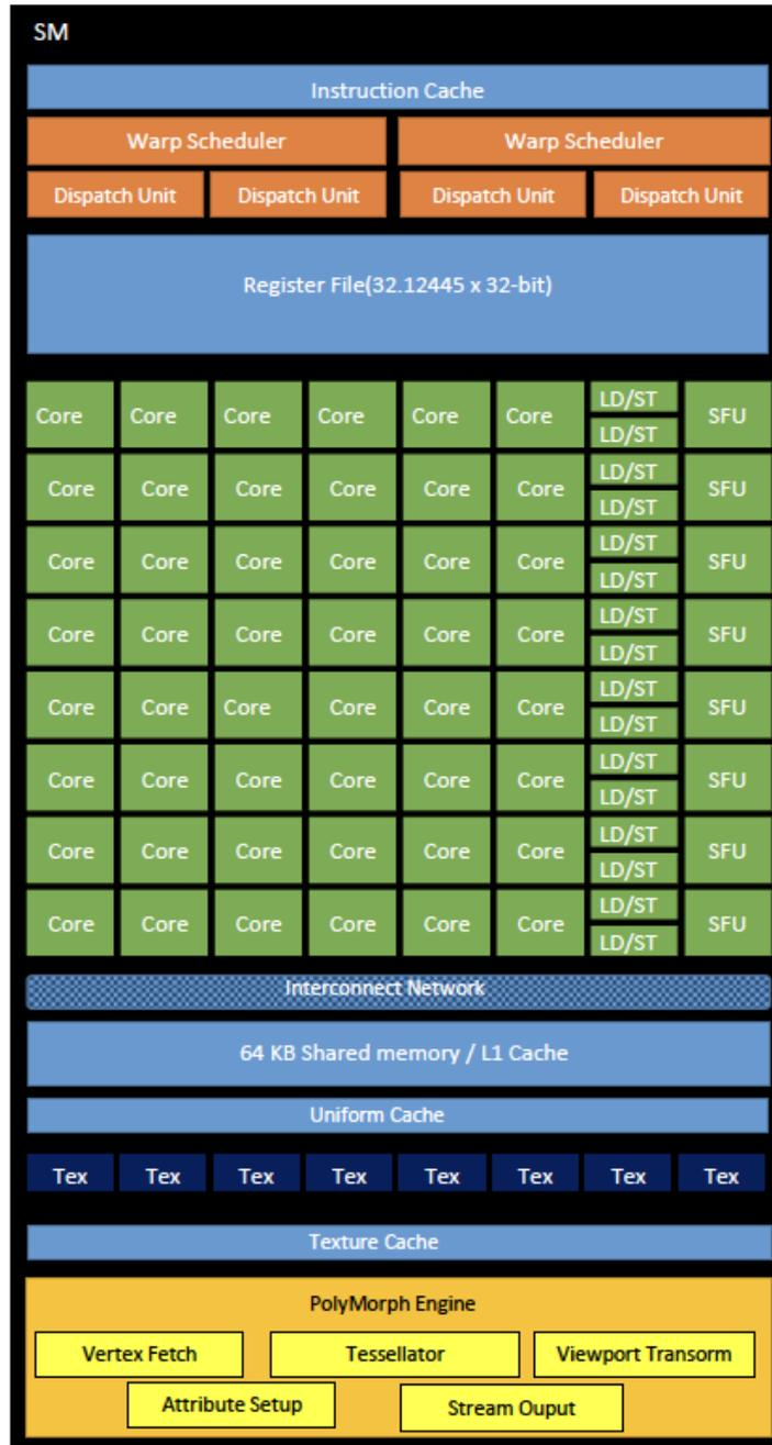
Figure 3.14. Example of an SM architecture (<https://www.geforce.com/hardware/desktop-gpus/geforce-gtx-580/architecture>).
