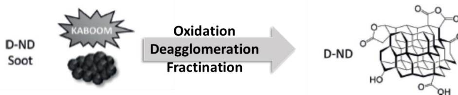
Figure 1.8: Illustration of the synthesis and post-synthetic treatment in the preparation of D-NDs (image is taken from ref [85]).
