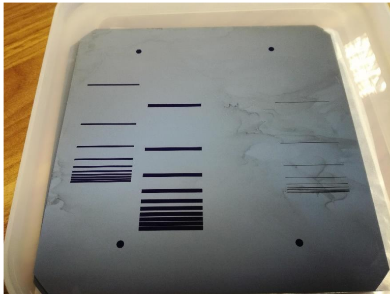
Figure 66: Picture of a sample with completely removed hot-melt after 1.5 minute in KOH free etchant with ultrasounds (35kHz)
