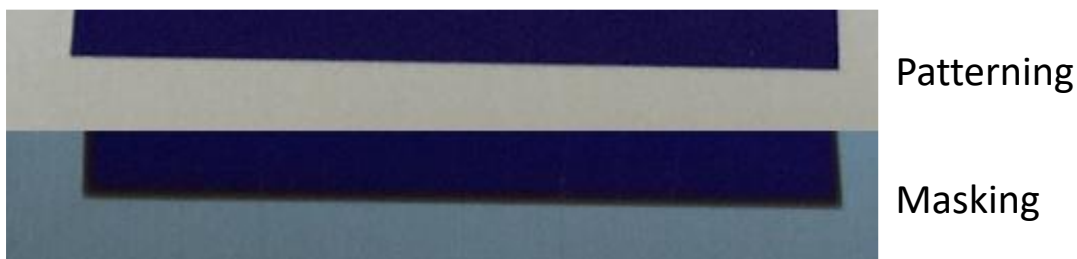
Figure 71: Pattern edges: sharp aspect using patterning technique (top) and blurred aspect using masking technique (bottom). Both lengths measure approximately 2cm
