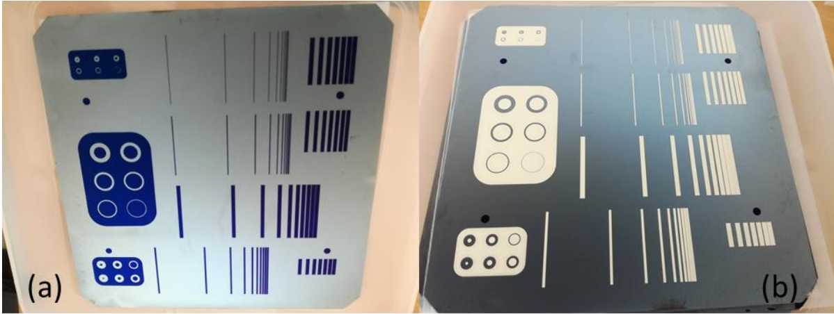
Figure 69: Picture of TLM samples (a) after hot-melt removal (same as Figure 63(b)) and (b) after aligned screen-print. The dots are used as alignment marks
