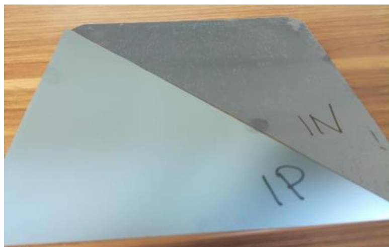
Figure 65: Picture with two samples after KOH etching, with IN side (top-right half) appearing visibly degraded with white dots, and IP sample (bottom-left) appearing unaffected
