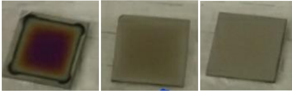
Figure 94: \text{La}_2\text{CuO}_4 over ZnO (400nm thickness) with Si substrate for a) 5000 pulses, b) 3000 pulses, c) 1000 pulses.
