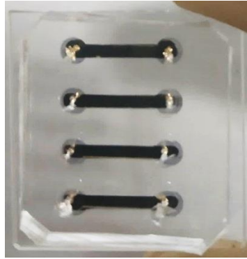
Figure 6.2 4 channel Ag/Au sensor (here with fluidic facilities).
