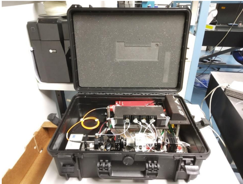
Figure P.1 Portable SPR system developed by project partner MULTITEL.
