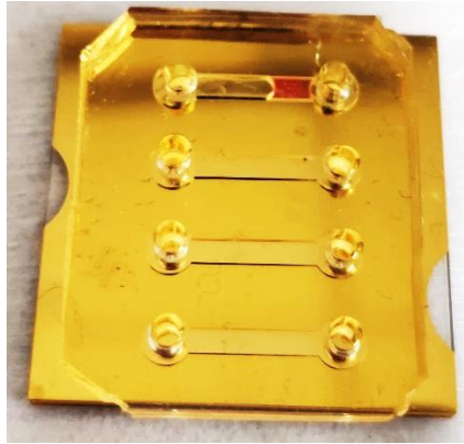
Figure 3.4 Au plasmonic sensor with microfluidic PDMS channels.
