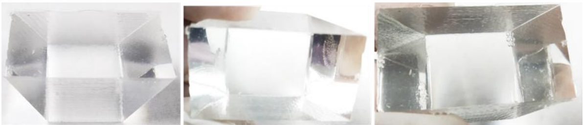
Figure 5.13 Fabricated PDMS prism.
