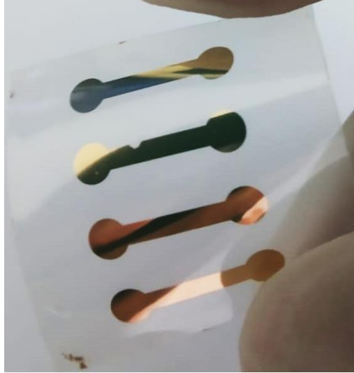
Figure 5.22 Flexible 4 channel tape sensor.
