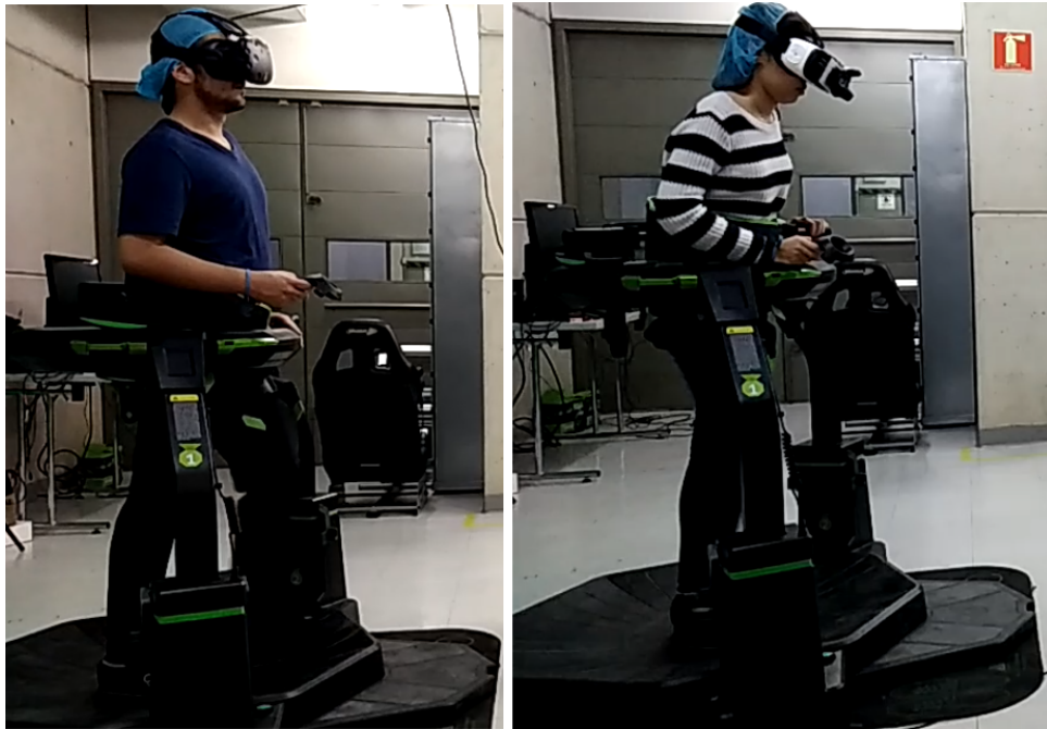
Figure 3.6: Blind-walking-tests using the Virtuix Omni treadmill
