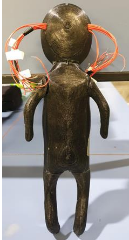
Figure 5.2: Preterm thermal manikin assembled after instrumenting with the heating wires. The cables connecting the heating wires to the power supply (in orange) are leaving through the head at the ear sides.
