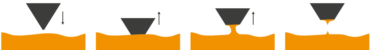
Figure 4.23: Plunging the tip. The tip is plunged of several tens of nanometers into gold. When withdrawn, some gold picked up by the tip creates a new pristine apex.
