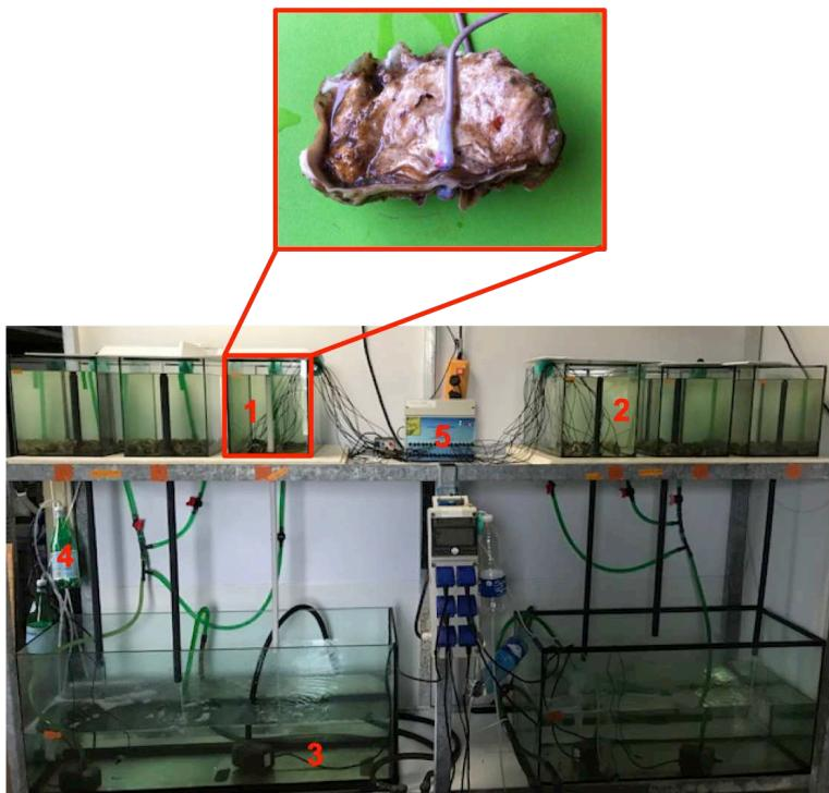
**Fig. S1.** Experimental design located in an experimental laboratory (LIENSs La Rochelle – CNRS). The numbers correspond to: (1) experimental batch of exposed oysters equipped with valvometric electrodes (zoom picture), (2) second experimental batch of exposed oysters, (3) buffer tank, (4) reduced vibrations thanks to the capacitance chamber and (5) HFNI valvometer (High Frequency Non-Invasive) connected to the electrodes stuck on oysters.
