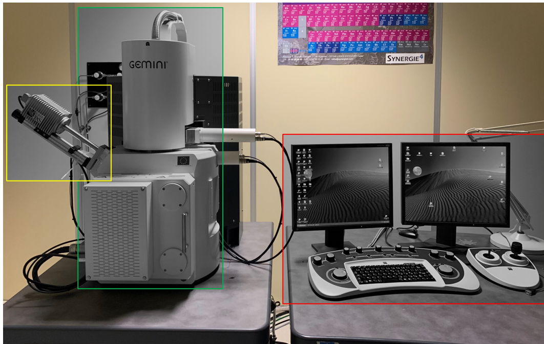
Figure 2.22 – Gemini SEM by Zeiss. Microscope (green box), EDX (yellow box), controllers (red box).
