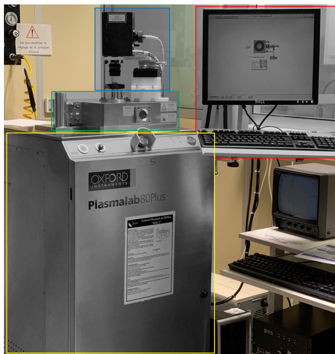
Figure 2.11 – Oxford Instruments Plasmalab 80 Plus RIE. Main chamber (green box), pumps and electronics (yellow box), interferometer (blue box) and controller (red box).
