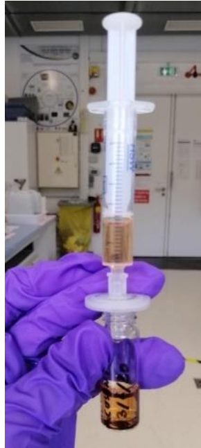
Figure 11. Filtration of a solution containing a mixture of myoglobin and COSAN using cellulose acetate 0.2 \mu\text{m} filter.
