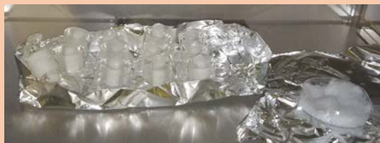
Protocol Figure 2.3. Optical image of the fabrication of the porous PDMS inside the vacuum oven.
