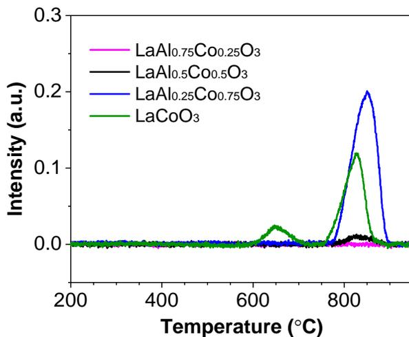
**Figure 3.4-** O<sub>2</sub>-TPD profiles of LaCo<sub>1-x</sub>Al<sub>x</sub>O<sub>3</sub> samples calcined at 700 °C.
