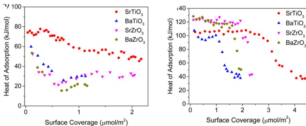
**Figure 1.13-** Heat of adsorption of (left)  $\text{NH}_3$  and (right)  $\text{CO}_2$  on perovskite catalysts <sup>166</sup>.
