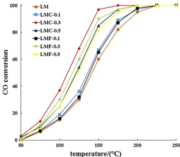
**Figure 1.15** - CO oxidation over  $\text{LaMn}_{1-x}\text{B}_x\text{O}_3$  ( F=Fe; M=Mn; C=Cu)<sup>178</sup>.
