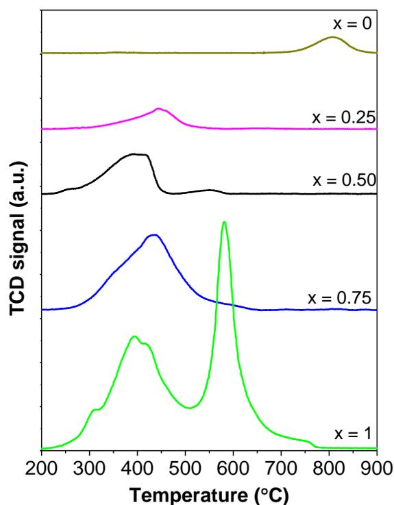
**Figure 3.3** – H<sub>2</sub>-TPR profiles of the samples LaAl<sub>1-x</sub>Co<sub>x</sub>O<sub>3</sub> calcined at 700 °C.
