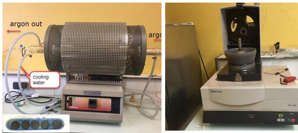
**Figure 2.1** – The Ar-flow furnace setup for LaSrCoO<sub>4</sub> synthesis and mortar pestle machine.
