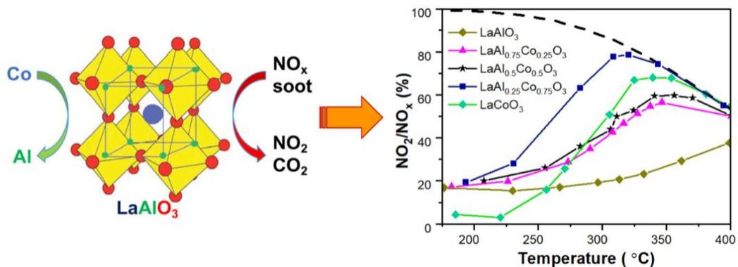
**Figure 2** – Catalytic application of LaAl<sub>1-x</sub>Co<sub>x</sub>O<sub>3</sub> for NO<sub>x</sub> – assisted soot oxidation.
