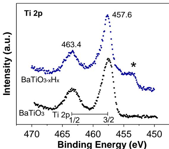
Figure 4.14 – Ti 2p XPS profiles of  $\text{BaTiO}_3$  and  $\text{BaTiO}_{3-x}\text{H}_x$ .
