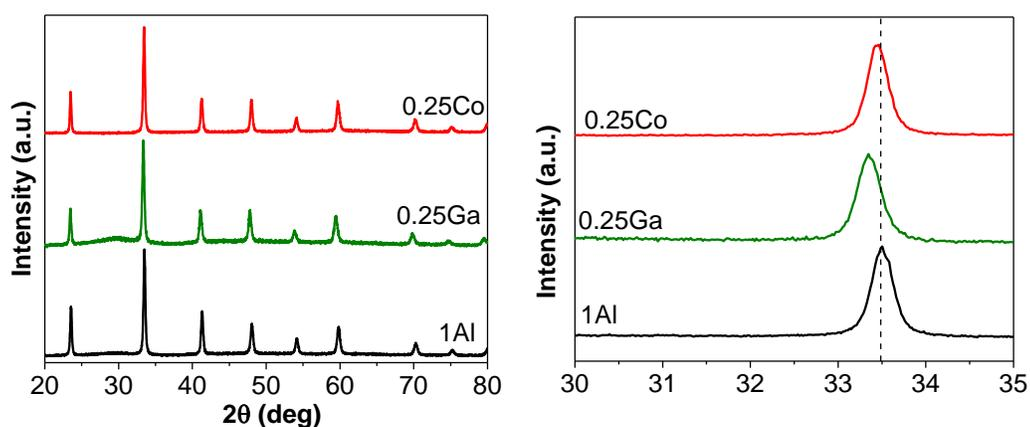
**Figure 5.1** – X-ray diffraction patterns of  $\text{LaAlO}_3$  (1Al),  $\text{LaAl}_{0.75}\text{Co}_{0.25}\text{O}_3$  (0.25Co) and  $\text{LaAl}_{0.75}\text{Ga}_{0.25}\text{O}_3$  (0.25Ga) and their magnifications.
