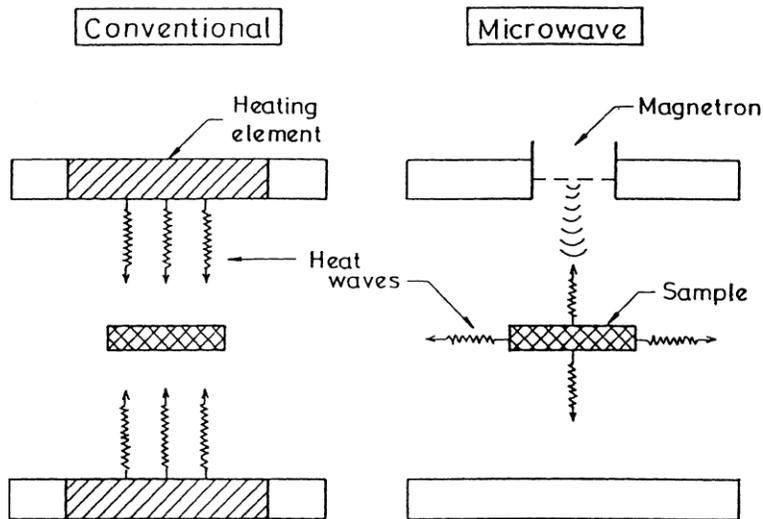
**Figure 1.2** – Principle of microwave heating vs conventional heating<sup>52</sup>.
