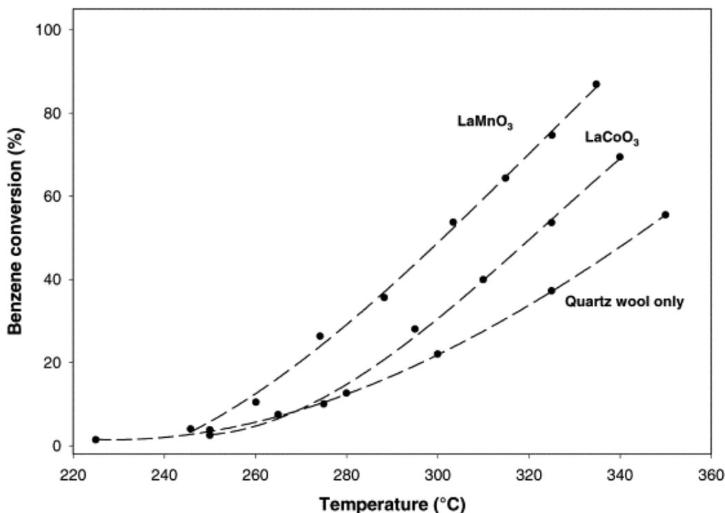
**Figure 1.17** – Benzene combustion over LaCoO<sub>3</sub> and LaMnO<sub>3</sub> <sup>187</sup>.
