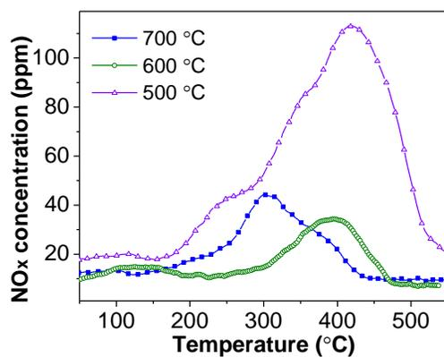
**Figure 3.12** - NO<sub>x</sub> desorption curves of LaAl<sub>0.25</sub>Co<sub>0.75</sub>O<sub>3</sub> calcined at different temperatures.
