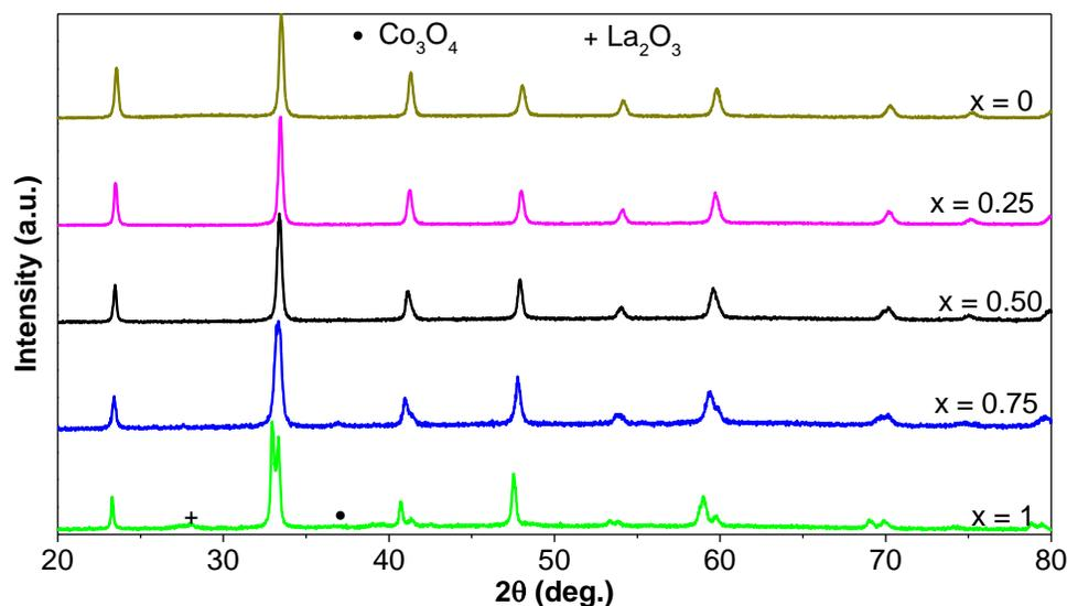
**Figure 3.1**– X-Ray diffractions of  $\text{LaAl}_{1-x}\text{Co}_x\text{O}_3$  calcined at 700 °C.
