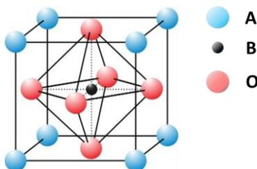
**Figure 1** – A model of perovskite structure  $ABO_3$ .
