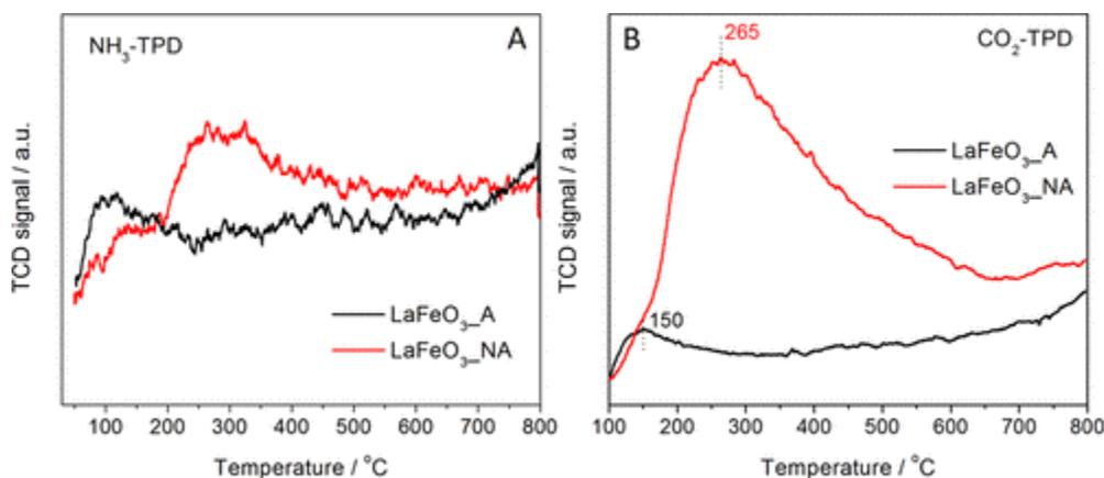
**Figure 1.11** - NH<sub>3</sub>-TPD (A) and CO<sub>2</sub>-TPD (B) results from LaFeO<sub>3</sub> prepared by carbon templating ( LaFeO<sub>3</sub>\_NA) and sol – gel (LaFeO<sub>3</sub>\_A) method <sup>162</sup>.
