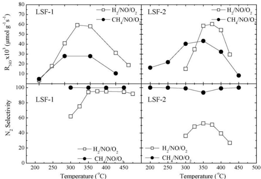
**Figure 1.21** – Temperature profiles of the rates of NO conversion and N<sub>2</sub> selectivity of CH<sub>4</sub>-SCR (NH<sub>4</sub>/NO/O<sub>2</sub>) and H<sub>2</sub>-SCR (H<sub>2</sub>/NO/O<sub>2</sub>). Reaction conditions (0.67 mol % CH<sub>4</sub> + 0.5 mol % NO + 5 % O<sub>2</sub> or 1 mol % H<sub>2</sub> + 0.5 mol % NO + 10 % O<sub>2</sub>)<sup>231</sup>.
