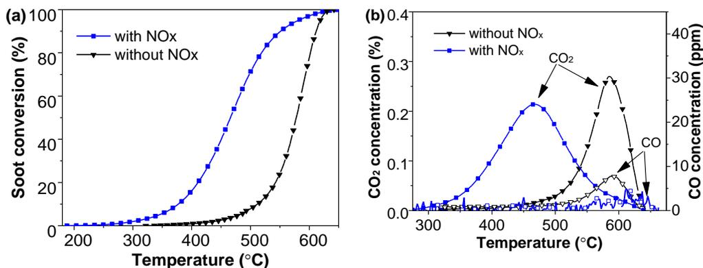
**Figure 3.8-** Soot conversion (a), CO<sub>2</sub> and CO concentration (b) as functions of temperature during soot oxidation catalytic tests with and without NO<sub>x</sub> supply over LaAl<sub>0.25</sub>Co<sub>0.75</sub>O<sub>3</sub> catalyst.
