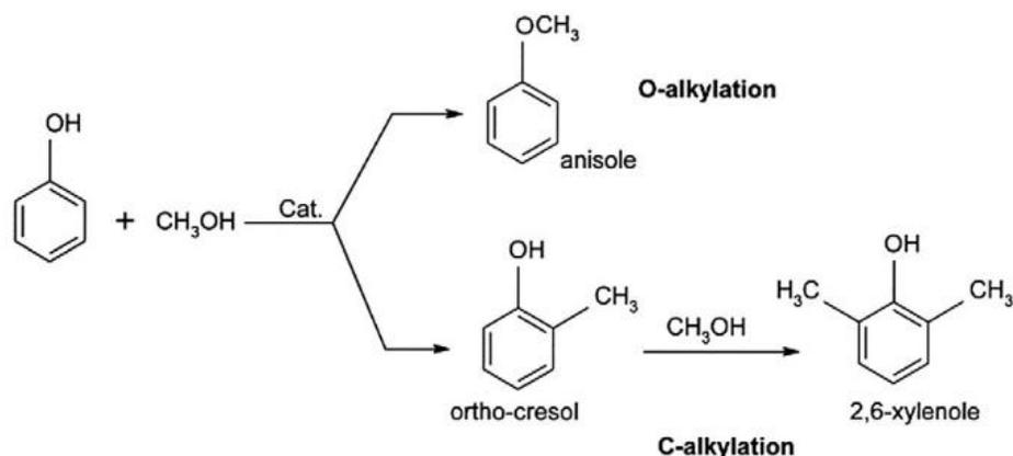
**Figure 1.25**– Main reaction pathway of phenol methylation<sup>242</sup>.
