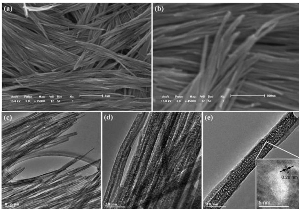
**Figure 1.4** – SEM (a,b) and TEM (c,d,e) images of mesoporous  $\text{SrTiO}_3$  nanowires<sup>93</sup>.
