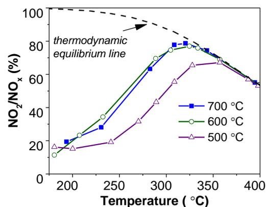
**Figure 3.13** - NO<sub>2</sub> percentage of LaAl<sub>0.25</sub>Co<sub>0.75</sub>O<sub>3</sub> calcined at different temperatures.
