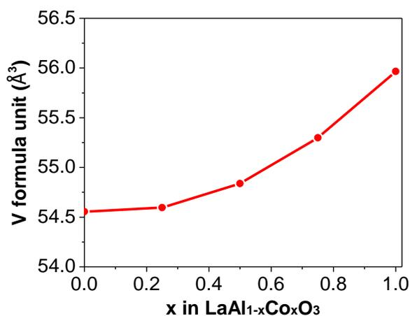
**Figure 3.2** –Volume of the formula units LaAl<sub>1-x</sub>Co<sub>x</sub>O<sub>3</sub> as a function of the cobalt fraction.
