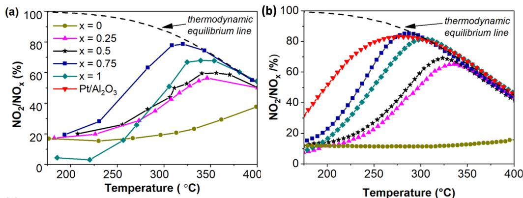
**Figure 3.7** – NO<sub>2</sub> percentage of LaAl<sub>1-x</sub>Co<sub>x</sub>O<sub>3</sub> calcined at 700 °C in (a) steady state conditions and (b) dynamic conditions.
