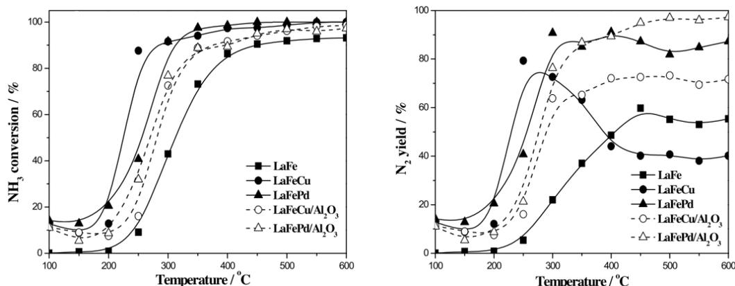
Figure 1.19 -  $\text{NH}_3$  conversion and  $\text{N}_2$  yield over different perovskite:  $\text{LaFeO}_3$  (LaFe);  $\text{LaFe}_{0.8}\text{Cu}_{0.2}\text{O}_3$  (LaFeCu);  $\text{LaFe}_{0.95}\text{Pd}_{0.05}\text{O}_3$  (LaFePd);  $\text{LaFe}_{0.8}\text{Cu}_{0.2}\text{O}_3$  supported on  $\text{Al}_2\text{O}_3$  (LaFeCu/ $\text{Al}_2\text{O}_3$ ) and  $\text{LaFe}_{0.95}\text{Pd}_{0.05}\text{O}_3$  supported on  $\text{Al}_2\text{O}_3$  (LaFePd/ $\text{Al}_2\text{O}_3$ )<sup>194</sup>.
