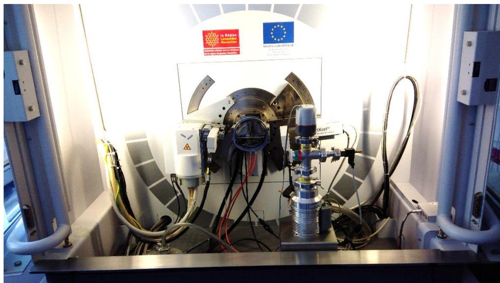
**Figure 2.4**– Empyrean PANalytical diffractometer for in-situ XRD experiments
