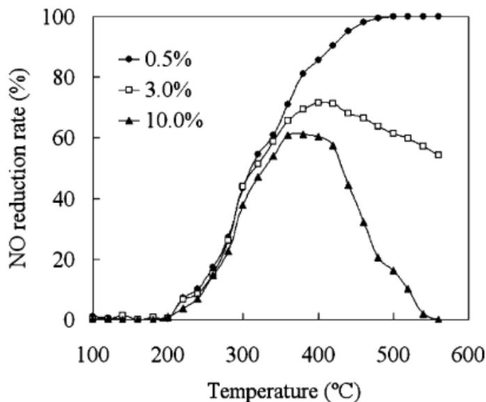
**Figure 1.22** - NO reduction curves under various O<sub>2</sub> concentrations over the La<sub>0.7</sub>Sr<sub>0.3</sub>MnO<sub>3</sub><sup>233</sup>.
