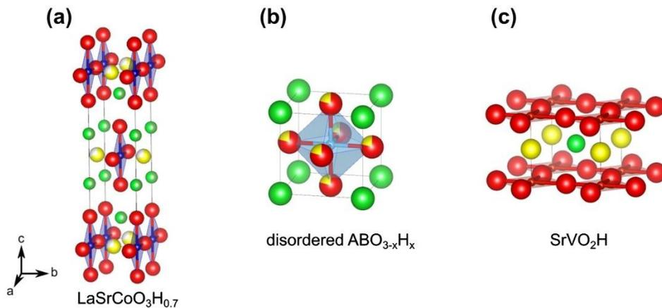
**Figure 4.1** – Some structures of oxyhydride perovskites: hydride is shown by yellow spheres and oxide is shown by red spheres; La and Sr cations are shown by shades of green <sup>25</sup>.
