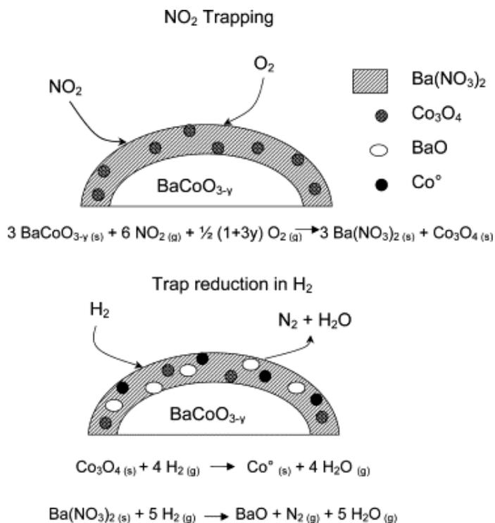
**Figure 1.20** - Scheme for the NO<sub>x</sub> trapping-regeneration process with the BaCoO<sub>3-y</sub> perovskite<sup>216</sup>.
