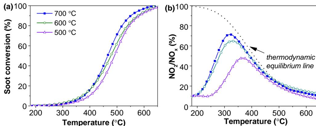
**Figure 3.14-** Soot oxidation (a), NO<sub>2</sub> percentage (b) of LaAl<sub>0.25</sub>Co<sub>0.75</sub>O<sub>3</sub> calcined at different temperature.
