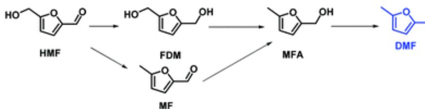
**Figure 1.26-** Possible reaction pathways for the hydrogenolysis of HMF <sup>21</sup>.
