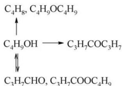
**Figure 1.24**– Reaction pathway of butanol-1 conversion<sup>240</sup>.
