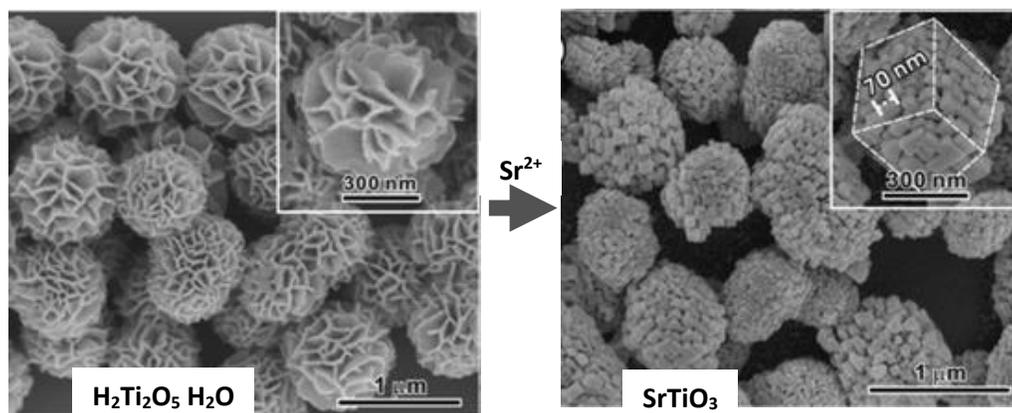
**Figure 1.3** – Flower-like protonated  $\text{TiO}_2$  precursor and its conversion to porous  $\text{SrTiO}_3$  by hydrothermal treatment with  $\text{Sr}^{2+}$ <sup>92</sup>.
