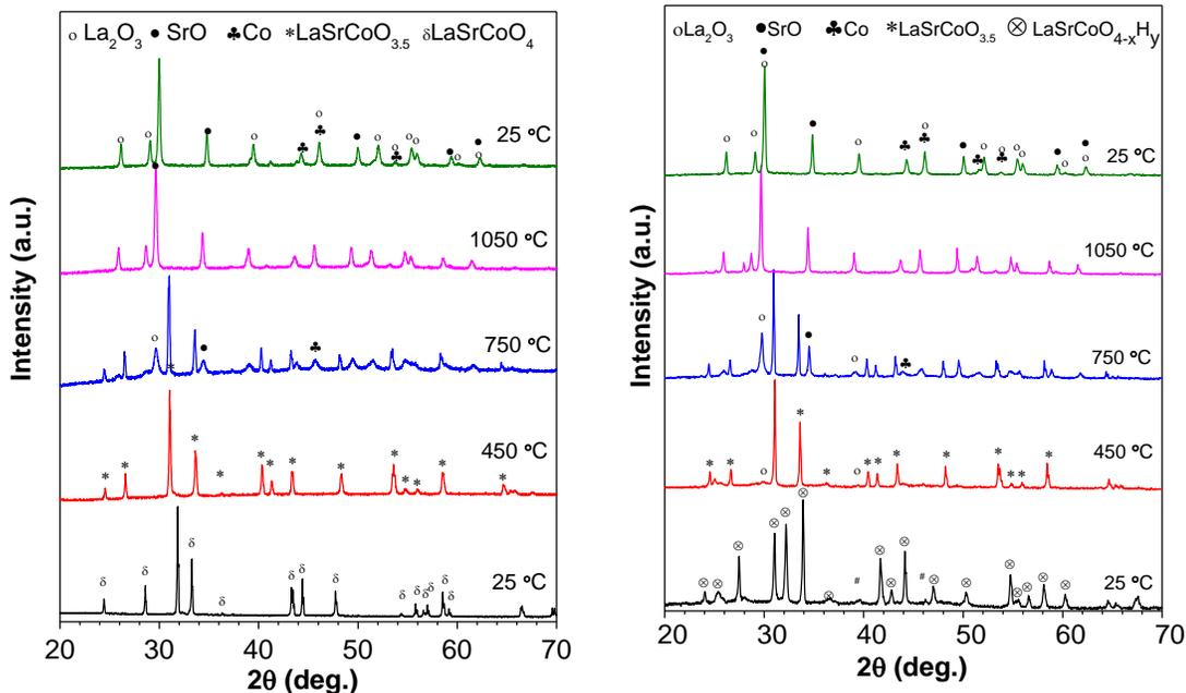
**Figure 4.10** – (a) In-situ X-ray diffractions of LaSrCoO<sub>4</sub> (left) and LaSrCoO<sub>4-x</sub>H<sub>y</sub> (right) under 5% H<sub>2</sub>/N<sub>2</sub>. La<sub>2</sub>O<sub>3</sub> (ICSD 01-073-2141), SrO (ICSD 00-048-1477) and metallic Co (ICSD 01-088-2325 and ICSD 00-015-0806). # stands for sample-Pt holder peaks.
