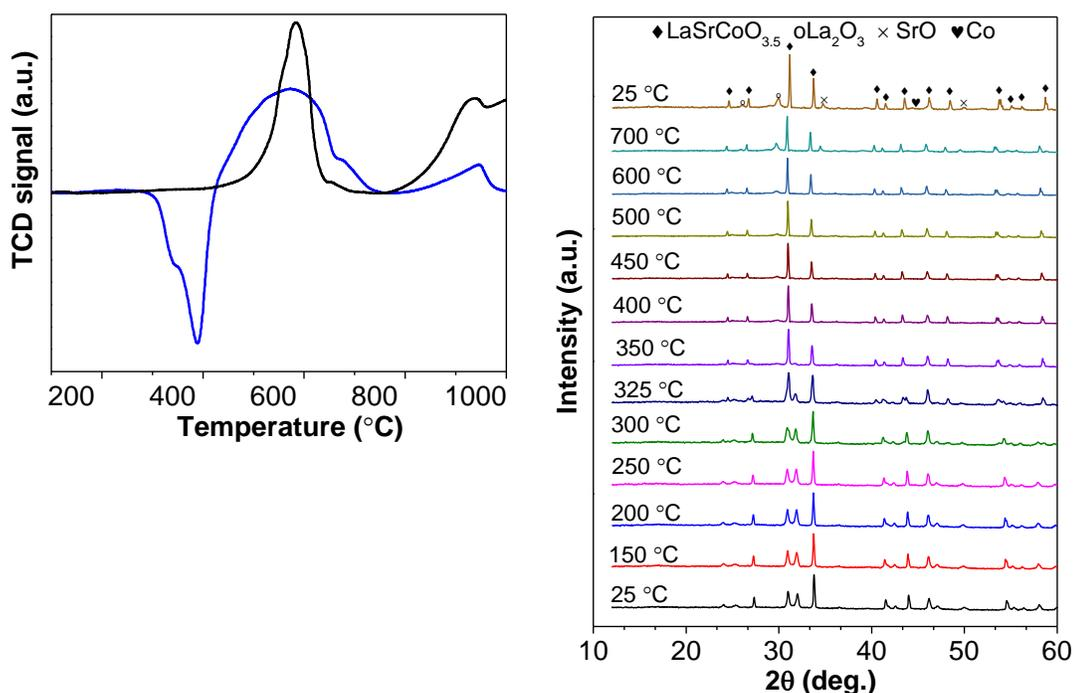
**Figure 4.12-** H<sub>2</sub>-TPR profile of LaSrCoO<sub>4-x</sub>H<sub>y</sub> (blue) and LaSrCoO<sub>4</sub> (black) in-situ XRD of LaSrCoO<sub>4-x</sub>H<sub>y</sub> under 5 %H<sub>2</sub>/N<sub>2</sub> at 5 °C.min<sup>-1</sup>; and *in-situ* XRD of LaSrCoO<sub>4-x</sub>H<sub>y</sub> under 5 %H<sub>2</sub>/N<sub>2</sub> at 5 °C min<sup>-1</sup>.
