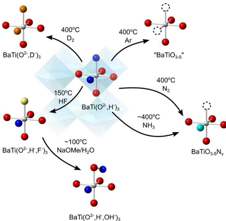
**Figure 4.2** - Anion exchange routes of BaTi(OH)<sub>3</sub><sup>25</sup>.
