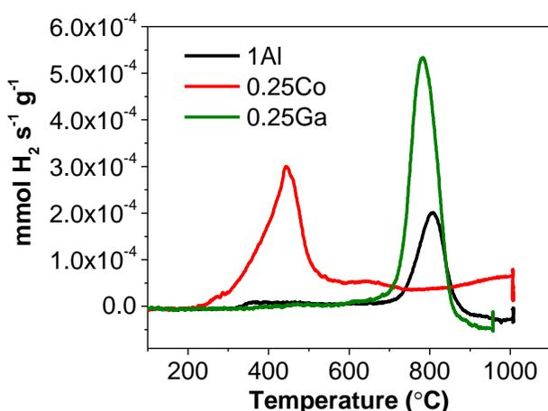
**Figure 5.3** -  $\text{H}_2$ -Temperature Reduction profiles of  $\text{LaAlO}_3$  (1Al),  $\text{LaAl}_{0.75}\text{Co}_{0.25}\text{O}_3$  (0.25Co) and  $\text{LaAl}_{0.75}\text{Ga}_{0.25}\text{O}_3$  (0.25Ga) (Samples were pretreated at  $500^\circ\text{C}$  under  $\text{N}_2$  in 30 min)
