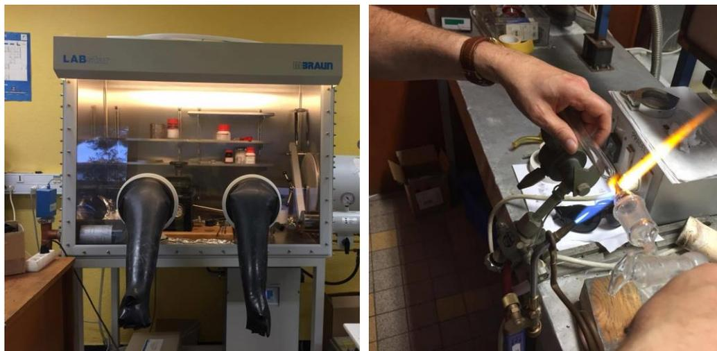
**Figure 2.2** – Argon glovebox and a flame sealed tube.
