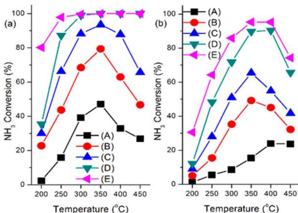
**Figure 1.18** - NH<sub>3</sub> conversions of the La<sub>1-x</sub>Sr<sub>x</sub>MnO<sub>3</sub> under (a) dry and (b) wet conditions in the range 200–450 °C. (A) Fresh catalyst, (B) 0.1h immersed in HNO<sub>3</sub>, (C) 1h- immersed in HNO<sub>3</sub>, (D) 10h- immersed in HNO<sub>3</sub>, and (E) 72h- immersed in HNO<sub>3</sub><sup>195</sup>.
