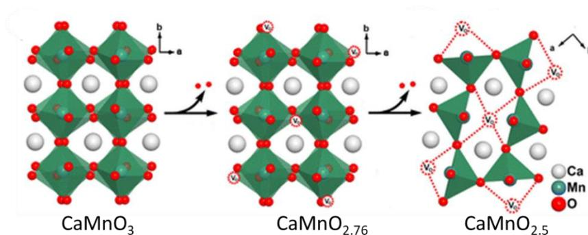
**Figure 1.6** - Structural transition from  $\text{CaMnO}_3$  to non-stoichiometric phases <sup>119</sup>.
