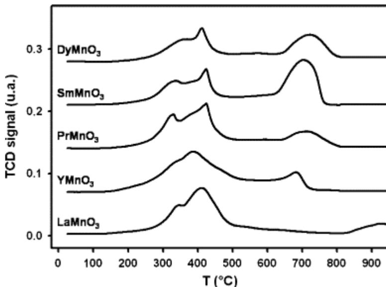
**Figure 1.8** – H<sub>2</sub> – TPR profiles of AMnO<sub>3</sub> perovskites <sup>139</sup>.
