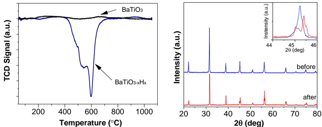
**Figure 4.9** - H<sub>2</sub>-TPR of profiles BaTiO<sub>3</sub> and the oxyhydride BaTiO<sub>3-x</sub>H<sub>x</sub> and XRD profiles after the experiment
