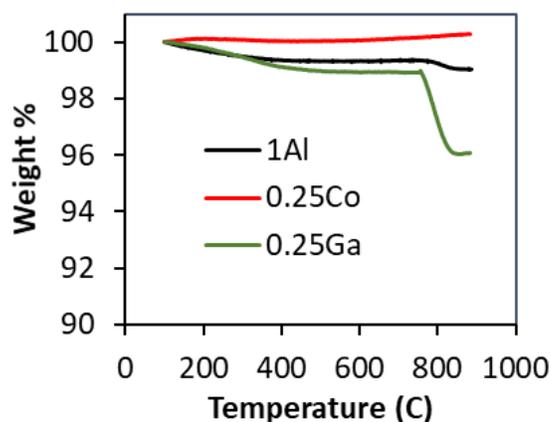
**Figure 5.4** - Thermal gravimetric analysis of the three catalysts
