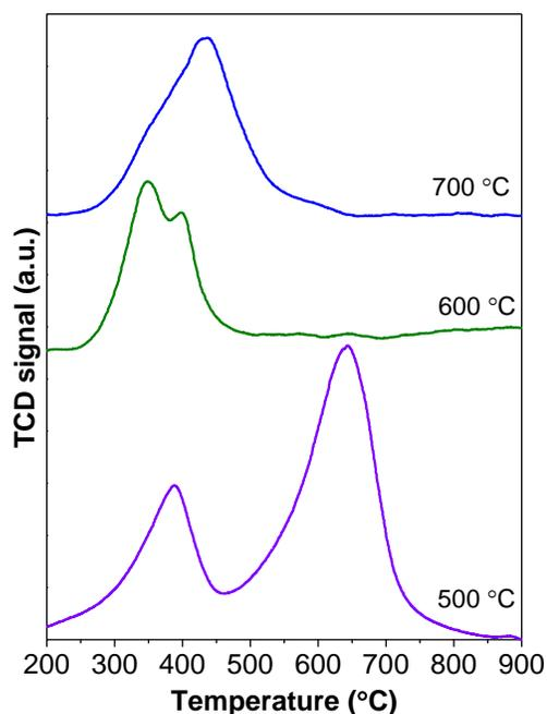
**Figure 3.11** – H<sub>2</sub>-TPR profiles of LaAl<sub>0.25</sub>Co<sub>0.75</sub>O<sub>3</sub> calcined at different temperatures
