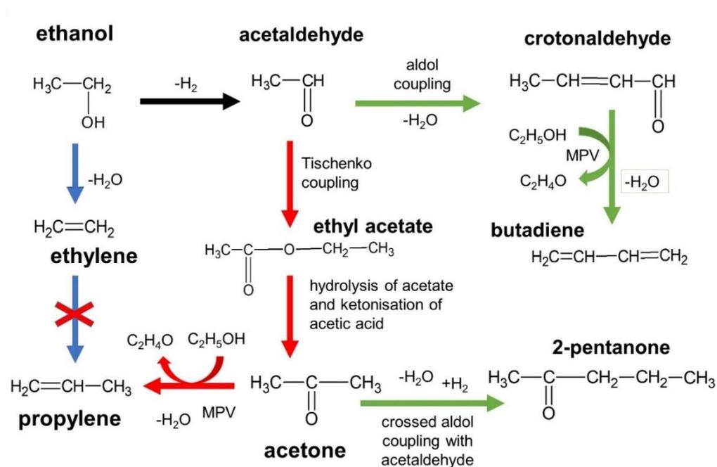
**Figure 4** - Main reaction pathways in the conversion of ethanol on Ga- and Co-doped LaAlO<sub>3</sub> perovskites.
