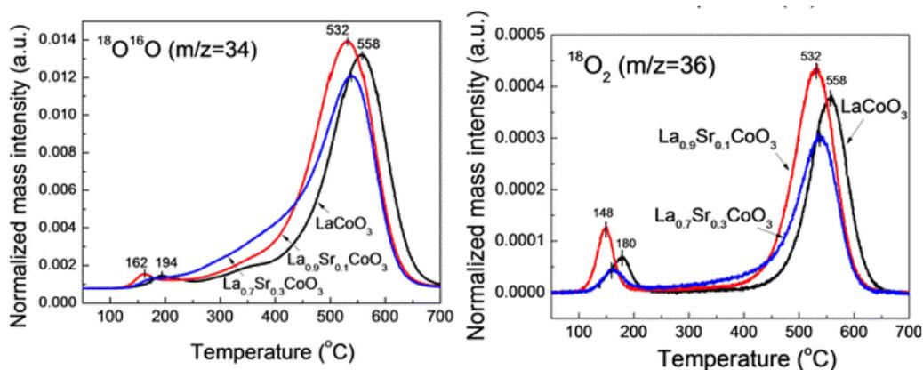
**Figure 1.10** - Changes in the (left) ( $^{18}\text{O}^{16}\text{O}$ ) and (right) ( $^{18}\text{O}_2$ ) signals for  $\text{La}_{1-x}\text{Sr}_x\text{CoO}_3$  catalysts pretreated with 1%  $^{18}\text{O}_2$  at 500  $^{\circ}\text{C}$  for 1 h as a function of temperature <sup>155</sup>.
