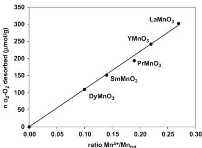
**Figure 1.9** – Correlation between  $\alpha_2$ -oxygen desorbed and the amount of  $\text{Mn}^{4+}$  in the  $\text{AMnO}_4$  perovskite structure <sup>139</sup>.
