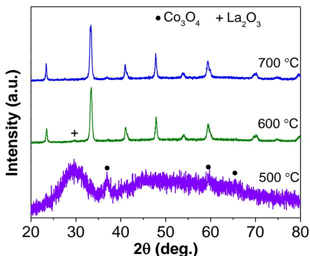
**Figure 3.10** - Diffraction patterns of LaAl<sub>0.25</sub>Co<sub>0.75</sub>O<sub>3</sub> calcined at different temperatures.
