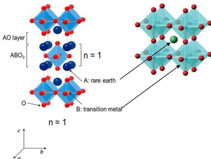
**Figure 1.1** - Perovskite oxides  $ABO_3$  and  $A_2BO_4$  structures
