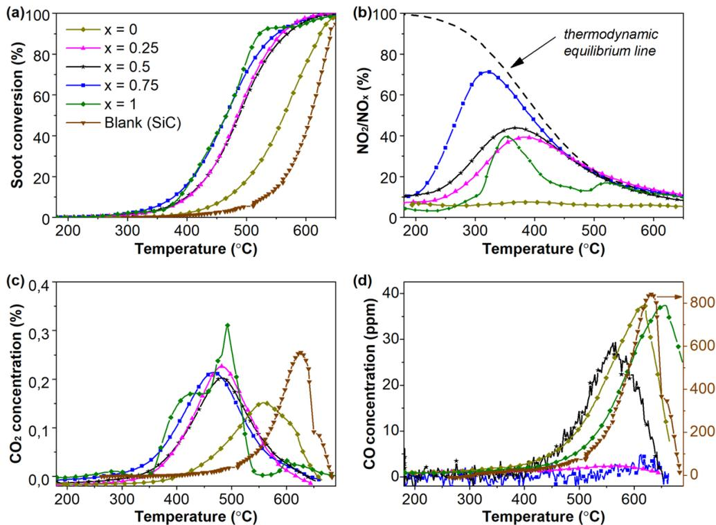
**Figure 3.9-** Soot oxidation (a), NO<sub>2</sub> percentage (b), CO<sub>2</sub> (c) and CO (d) concentrations (both Y axes) of  $\text{LaAl}_{1-x}\text{Co}_x\text{O}_3$  calcined at 700 °C.
