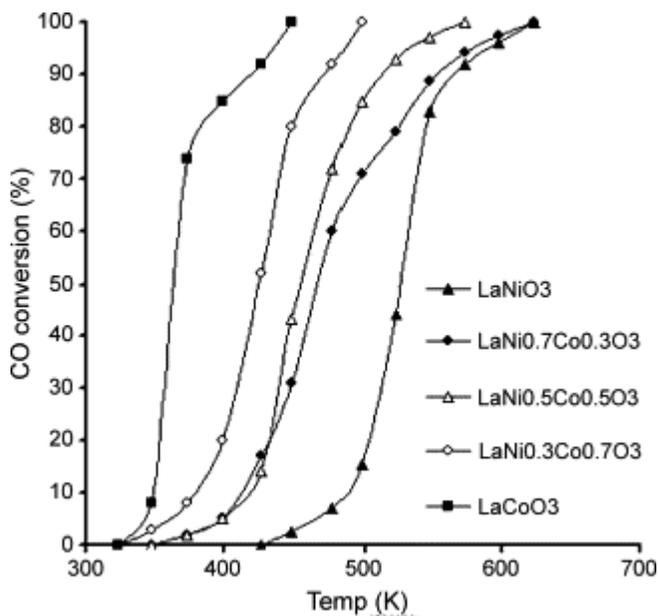
**Figure 1.14** - CO conversion as a function of catalyst temperature <sup>173</sup>.
