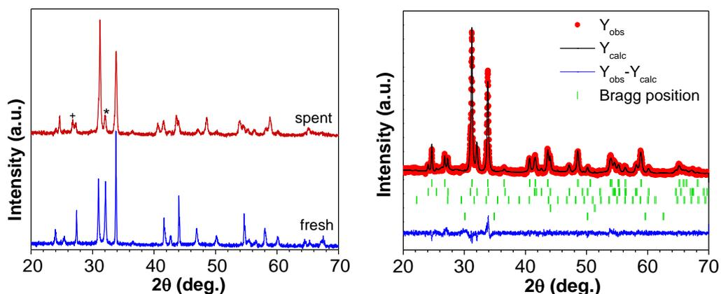
**Figure 4.20** - X-ray diffractions of fresh and spent LaSrCoO<sub>4-x</sub>H<sub>y</sub>, refinement of oxyhydride LaSrCoO<sub>4-x</sub>H<sub>y</sub> spent at 300 C of chemical titration (Bragg positions top to bottom: LaSrCoO<sub>3.5</sub>, LaSrCoO<sub>4-x</sub>H<sub>y</sub>, La<sub>2</sub>O<sub>3</sub>, Co and SrO).
