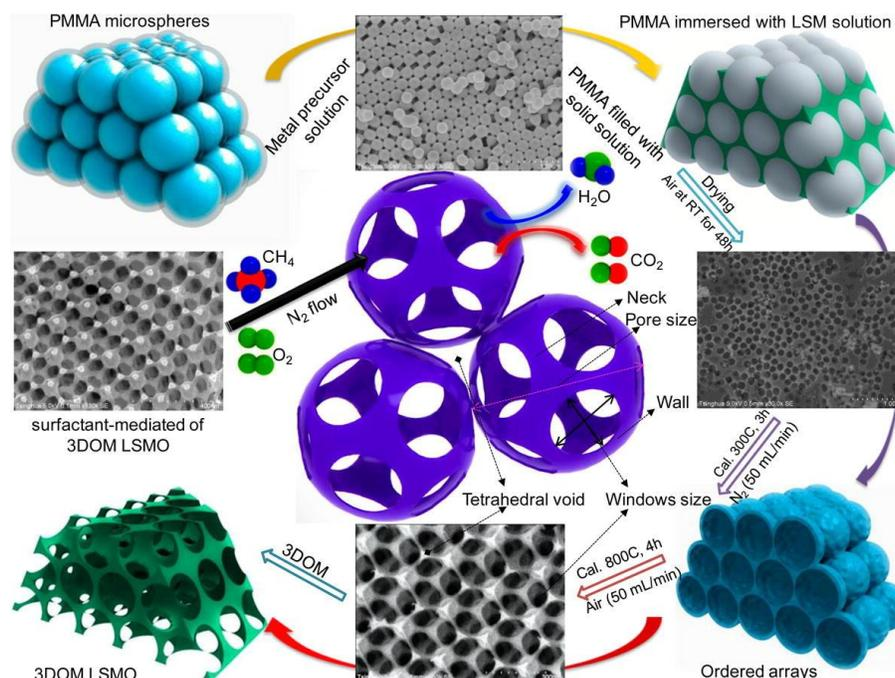
**Figure 1.5** - 3DOM La<sub>0.6</sub>Sr<sub>0.4</sub>MnO<sub>3</sub> perovskite prepared by the PMMA-templating method and its application for methane combustion <sup>108</sup>.
