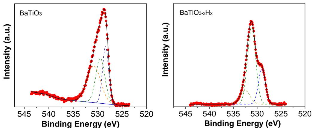
Figure 4.15 –  $\text{O}1s$  XPS profiles of  $\text{BaTiO}_3$  and  $\text{BaTiO}_{3-x}\text{H}_x$ .
