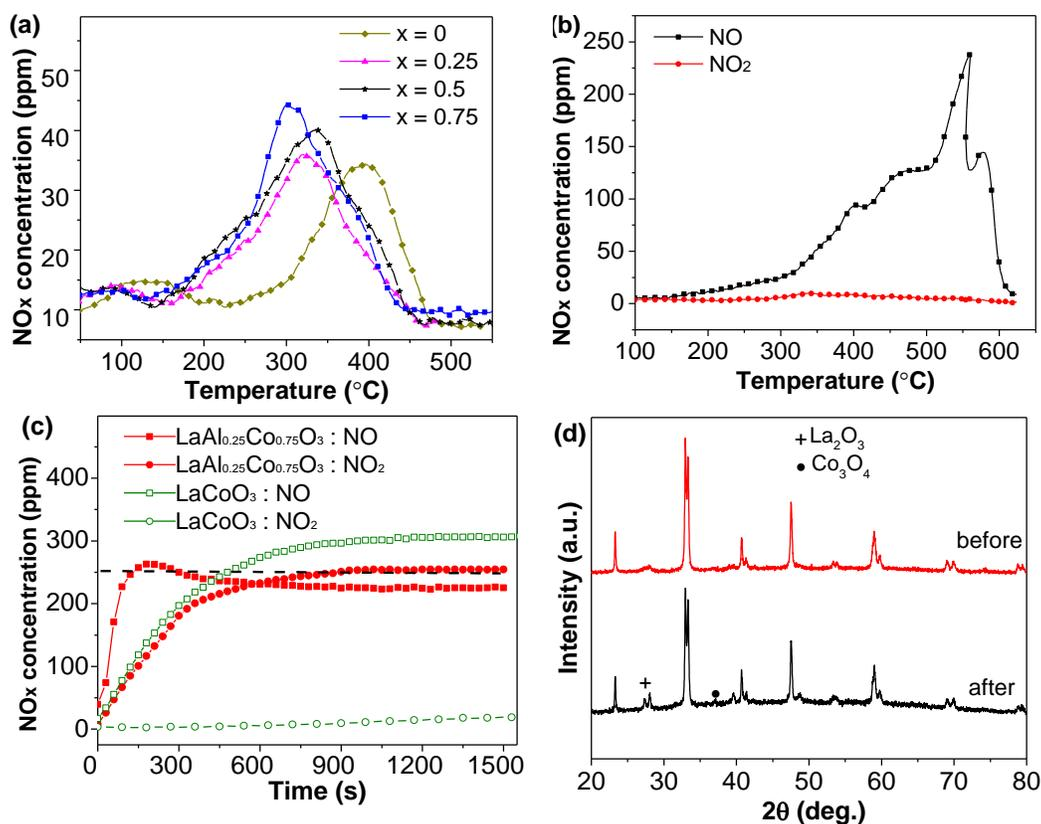
**Figure 3.6** – NO<sub>x</sub> desorption curves of LaCo<sub>1-x</sub>Al<sub>x</sub>O<sub>3</sub> calcined at 700 °C (a), NO<sub>x</sub> desorption of LaCoO<sub>3</sub> at 250 °C with time (b) (250 ppm of NO<sub>x</sub> and 250 ppm of NO<sub>2</sub> balance in N<sub>2</sub>; 250 °C); NO<sub>x</sub> adsorption on LaCoO<sub>3</sub> and LaAl<sub>0.25</sub>Co<sub>0.75</sub>O<sub>3</sub> at 250 °C (c), and XRD pattern of LaCoO<sub>3</sub> after the NO<sub>x</sub>-TPD experiment (d).
