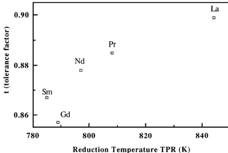
**Figure 1. 7** - Goldschmidt's tolerance factor  $t$  and reduction temperature obtained from temperature-programmed reduction experiments for the  $\text{LnCoO}_3$  perovskites <sup>132</sup>.
