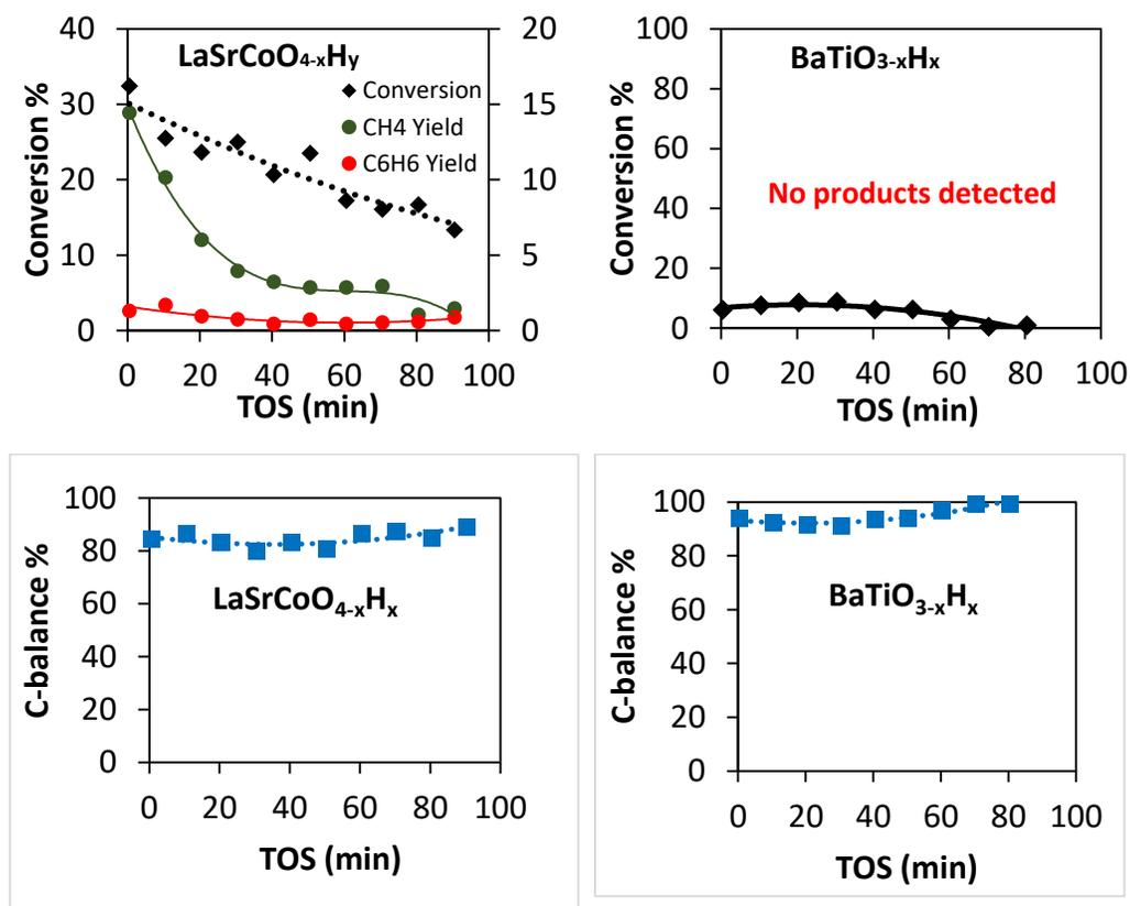
**Figure 4.18**– Toluene conversion and yields of products with time on stream of the chemical titration of oxyhydrides  $\text{LaSrCoO}_{4-x}\text{H}_y$  and  $\text{BaTiO}_{3-x}\text{H}_x$  (500 mg of the oxyhydride; 250 ppm of toluene in  $100 \text{ ml} \cdot \text{min}^{-1}$  of  $\text{N}_2$  flow at atmospheric pressure,  $T = 300 \text{ }^\circ\text{C}$ ); and C-balance
