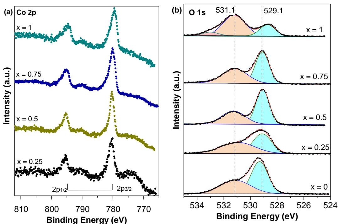
**Figure 3.5** – XPS spectra of Co 2p (a) and O 1s (b) of LaAl<sub>1-x</sub>Co<sub>x</sub>O<sub>3</sub>.
