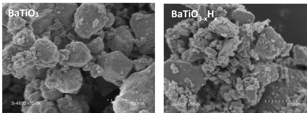
**Figure 4.13** - SEM images of  $\text{BaTiO}_3$  and  $\text{BaTiO}_{3-x}\text{H}_x$ .
