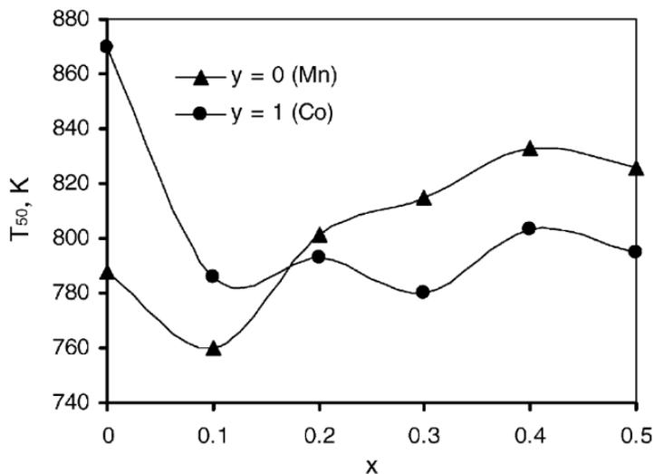
**Figure 1.16** – Temperatures of 50 % of conversion of methane to  $\text{CO}_2$  over  $\text{La}_{1-x}\text{Ce}_x\text{CoO}_3$  and  $\text{La}_{1-x}\text{Ce}_x\text{MnO}_3$  perovskites as a function of  $x$ <sup>186</sup>.
