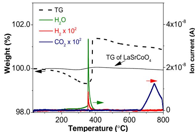
**Figure 4.7** - TGA-MS profile of  $\text{LaSrCoO}_{4-x}\text{H}_y$  under air.
