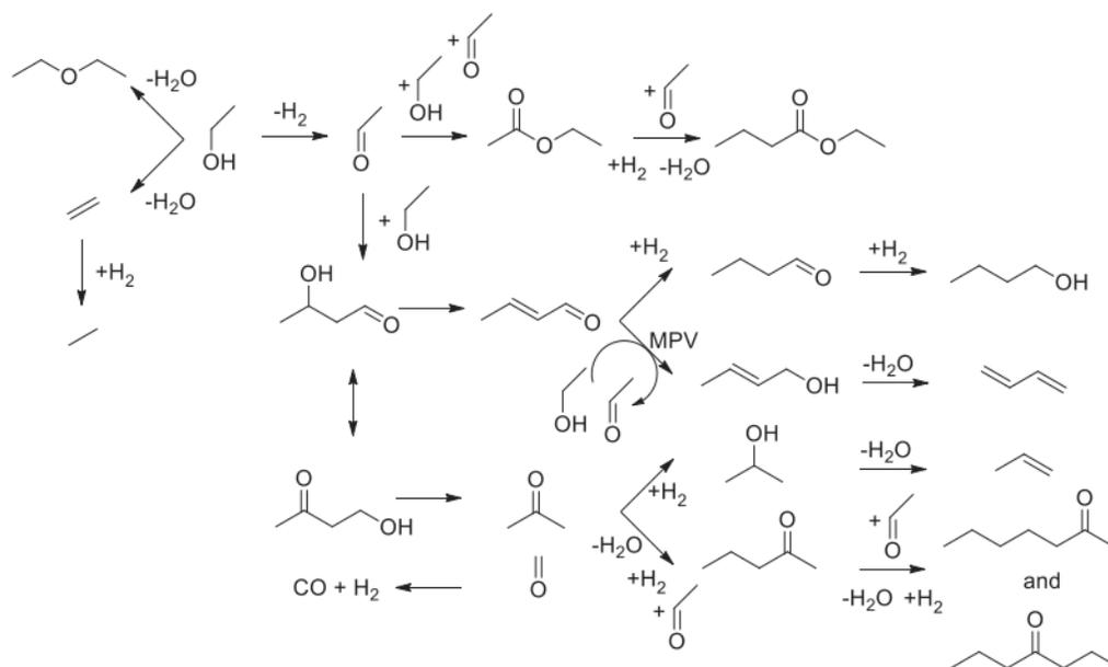
**Figure 1.23**– Generally accepted network of C – C coupling of ethanol<sup>239</sup>.
