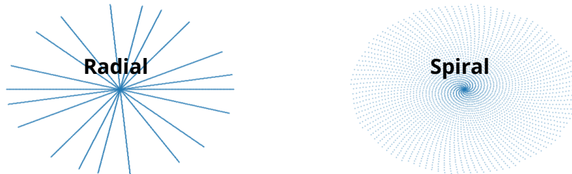
Figure 5.2-4: Schematic representation of the two multi-shot non-Cartesian (radial and spiral) readouts considered here for 2D imaging. In our setting, we used N_s = 100 shots, each of them consisting of 640 samples giving a total of m = 64,000 k-space measurements. Here only 10 shots are presented.
